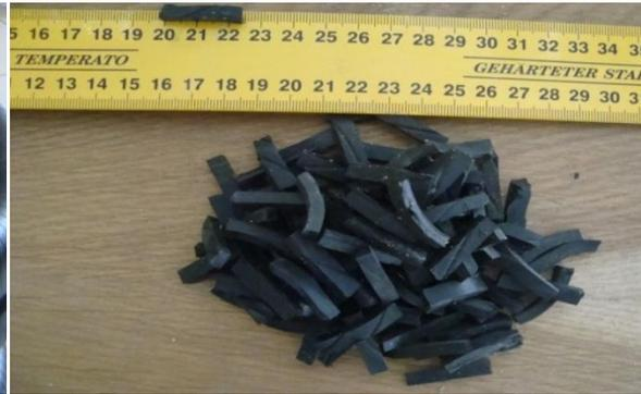
Figure 1.b.Rubber Aggregate (25 mm).
