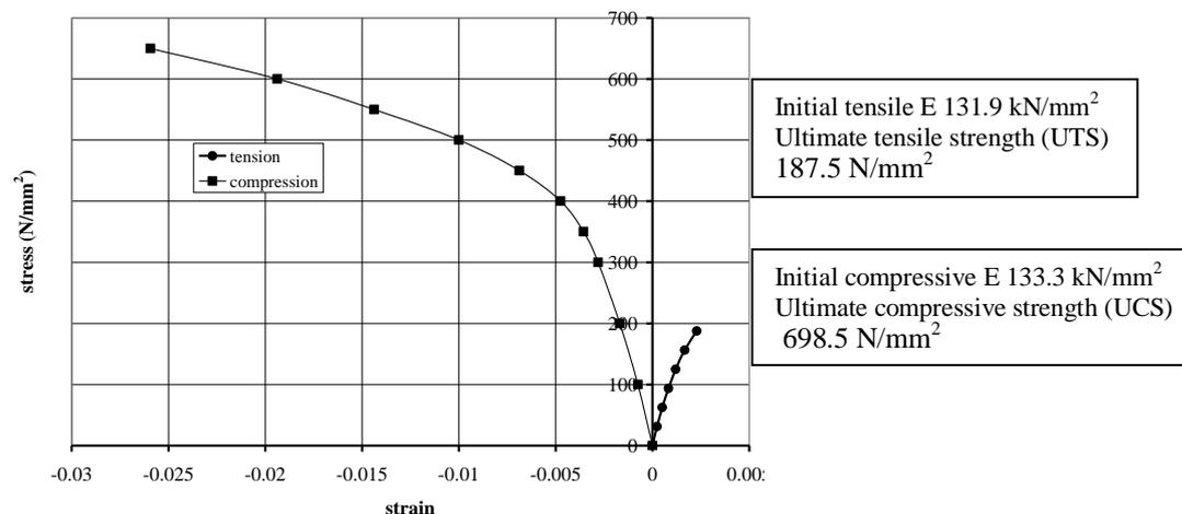
Figure 1. Typical stress-strain curves for early cast iron
