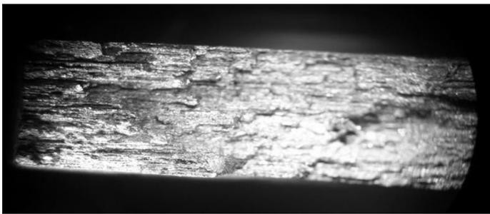
Figure 2. Photograph of tensile specimen failure surface showing the laminar structure of wrought iron
