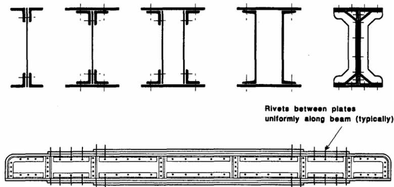
Figure 3. Typical cross-sections and elevation of wrought iron (Figures 3.7 and 3.8 in Bussell (1975))
