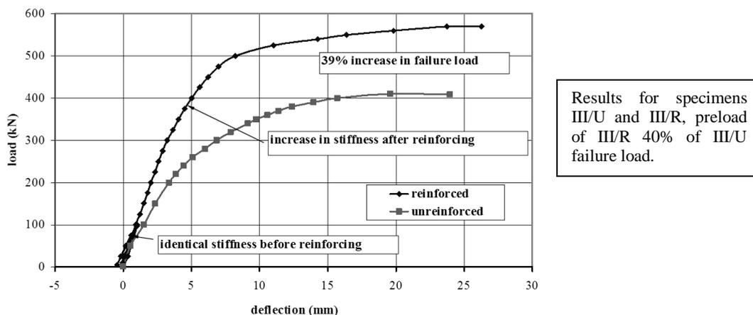
Figure 5. Graph showing benefits of CFRP strengthening, even under significant preload
