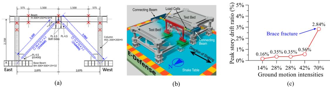
Figure 1. Two-third single-story chevron concentrically braced frame: (a) elevation view of test structure [adopted from Okazaki et al. (2013)]; (b) test-bed system [adopted from Okazaki et al. (2013)]; and (c) peak story drift ratios at various ground motion intensities.
