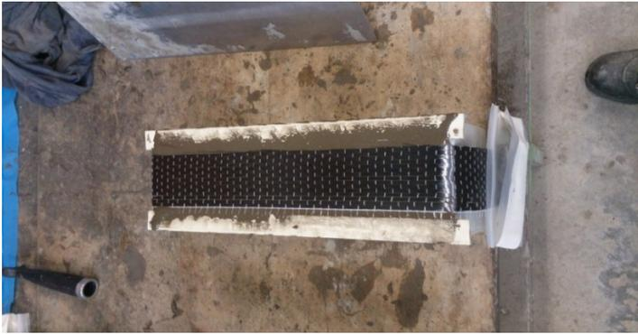
Figure 2. Bonding of CFRP fabric by geopolymer paste.
