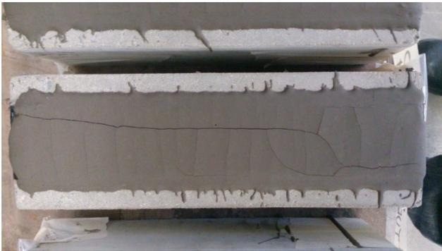
Figure 5. CFRP bonded to concrete by geopolymer paste.
