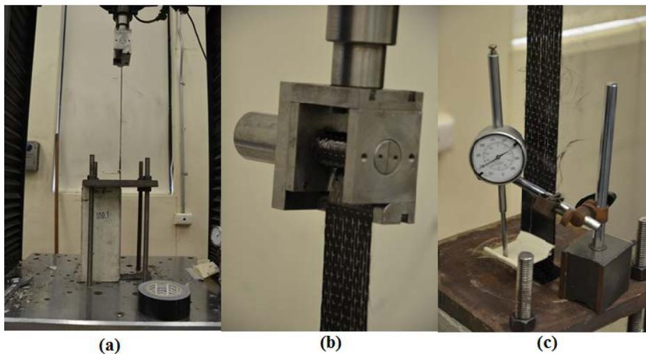
Figure 3. (a) Alignment and positioning of specimen, (b) Securing carbon fiber fabric to the grip for pull off, (c) Measurement of slip by dial gauge.
