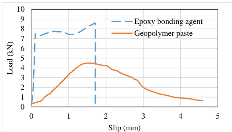
Figure 7. Load-slip curves of epoxy bonding agent and geopolymer paste.
