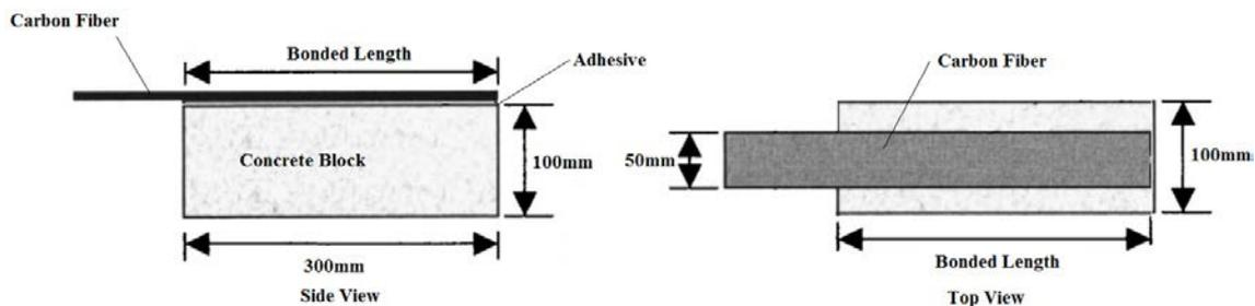
Figure 1. Specimens for bond test of CFRP fabric to concrete.
