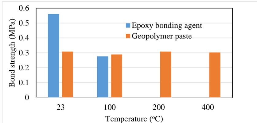
Figure 6. Bond strength of epoxy bonding agent and geopolymer paste.
