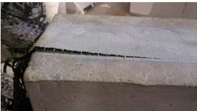
Figure 4. Delamination of epoxy bonded CFRP fabric by heat.
