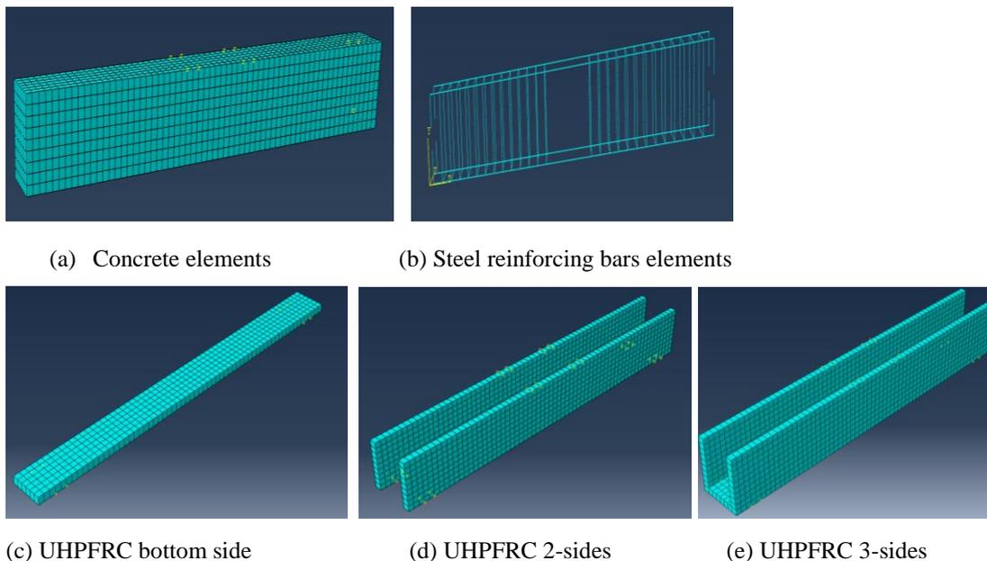
Figure 5: Meshed beam specimen
