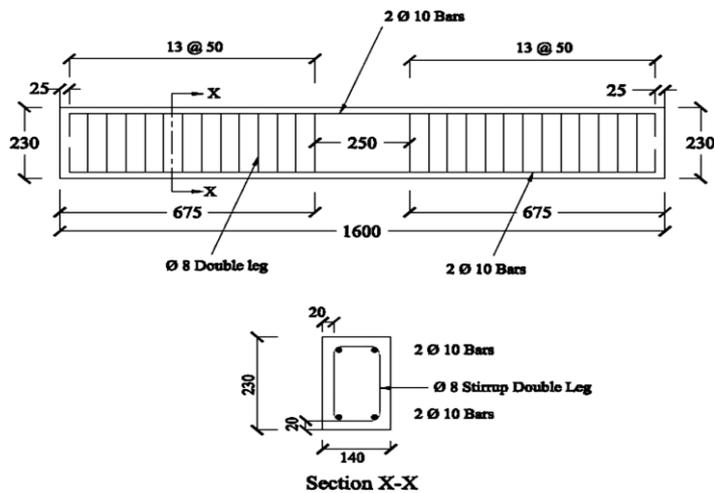
Figure 2. Geometry and details of concrete beam specimens (all dimensions in mm) (Al-Osta, Isa et al. 2017)
