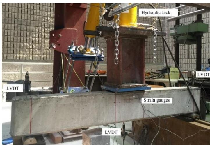
Figure 1: Beam test set-up
