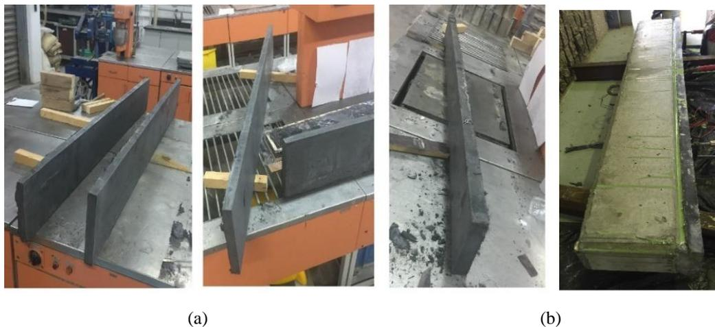
Figure 3: (a) UHPFRC strips (b) Strengthened beams specimens using epoxy adhesive bonding
