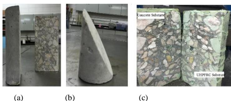
Figure 4: (a) Half split cylinders (b) Slant cut cylinders (c) Split cylinder tensile strength bond test
