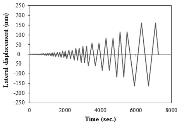
Figure 4. Loading regime for cyclic torsional loading
