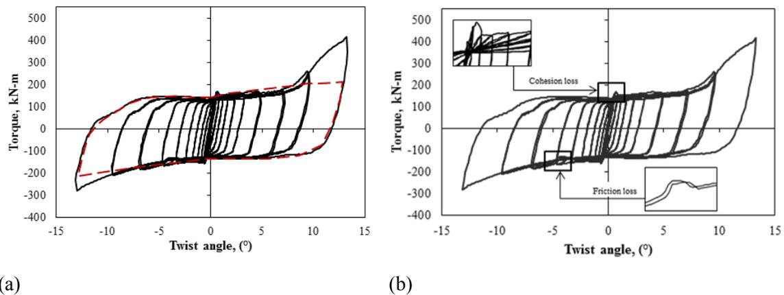
Figure 5. Torque-twist angle of HC-FCS column under pure torsion: (a) hysteretic with backbone curves, (b) cohesion and friction loss on the hysteretic curve
