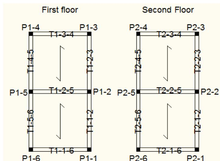
Figure 1. Plans of first and second floors with beams and columns identification label
