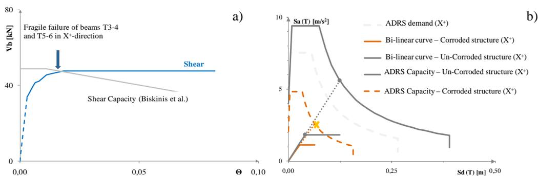
Figure 5. a) Shear failure according to Biskinis et al. (2004), b) ADRS representation of Push-over curves for un-corroded and corroded structure at third level of corrosion and second configuration  $X^+$ -direction.
