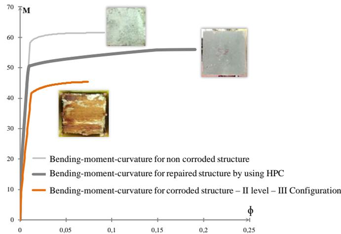
Figure 6. Bending moment-curvature graph in case of non corroded, corroded and retrofitted members
