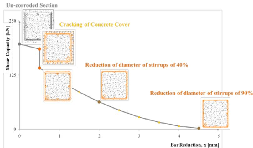
Figure 4. Corrosion Levels and correlation between shear capacity and bar reduction
