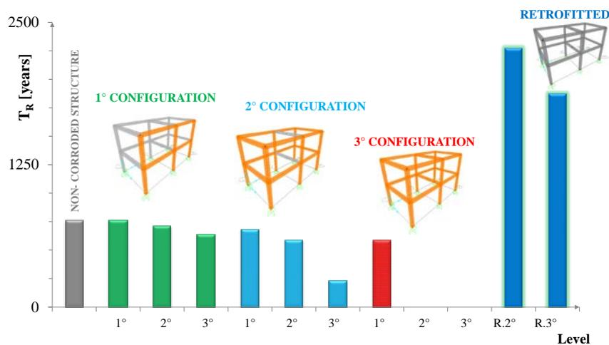
Figure 7. Corrosion levels and configurations related to Return period of seismic action yielding to lifesafe limit state for the structure
