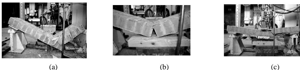
Figure 1. (a) Failure of specimen C1\_co due to fibres rupture, (b) Failure of specimens G3\_co due to fibres rupture, (c) Failure of specimen G7\_co due to shear diagonal tension.
