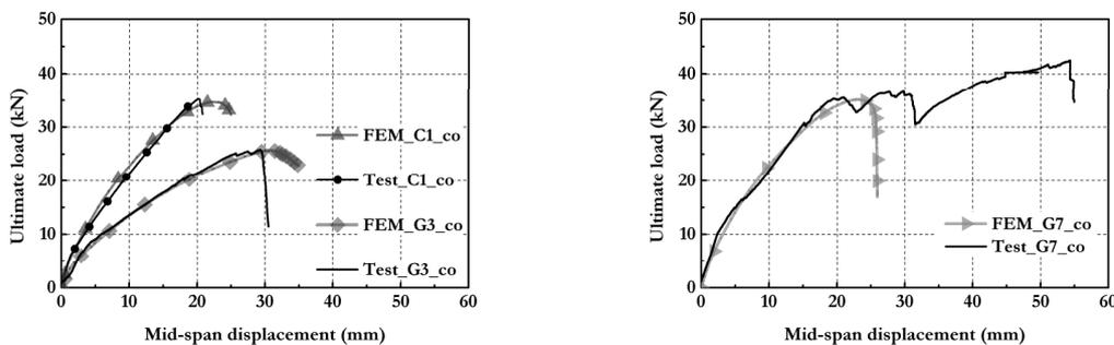
Figure 3. Finite element simulation results: Comparison against experimental results.
