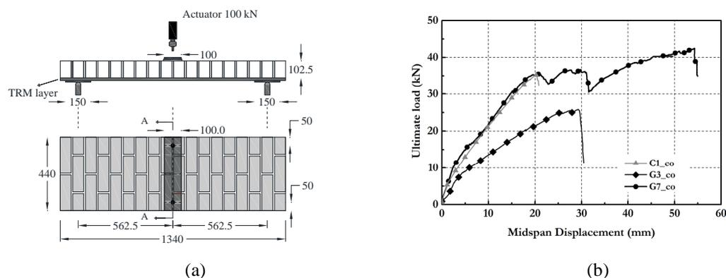
Figure 2. (a) Experimental setup (b) Experimental results: Load vs vertical deflection at mid-span curve
