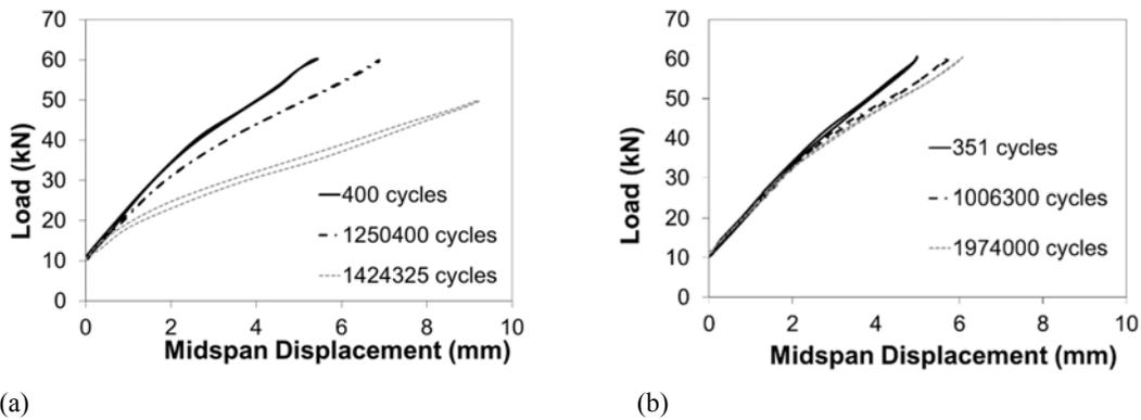
Figure 2. Stiffness degradation during fatigue testing (a) Beam B2: Freezing-thaw and fatigue (b) Beam B5: Fatigue only.
