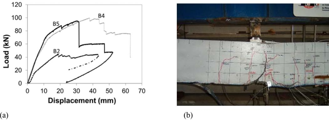
Figure 3. Static loading to failure (a) Load-deflection (b) Failure mode of Beam B5 (Photo: J. Ford).
