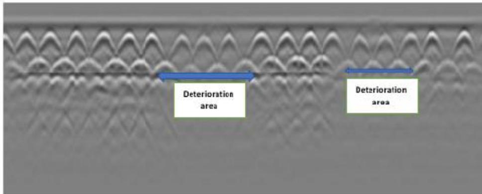
Fig. 7. Detection of deterioration areas in the image through visualization technique
