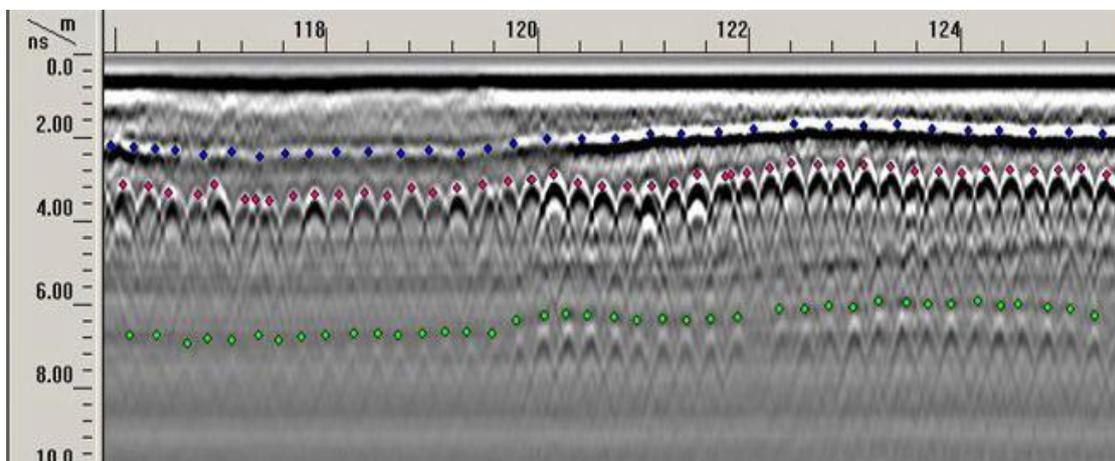
Fig. 1: GPR profile of a bridge deck in Queens, NY. The colored dots (blue – top of the slab, red – top reinforcing bar layer, and green – bottom reinforcing bar layer) indicate where amplitude measurements were taken (Tarussov et al, 2013)
