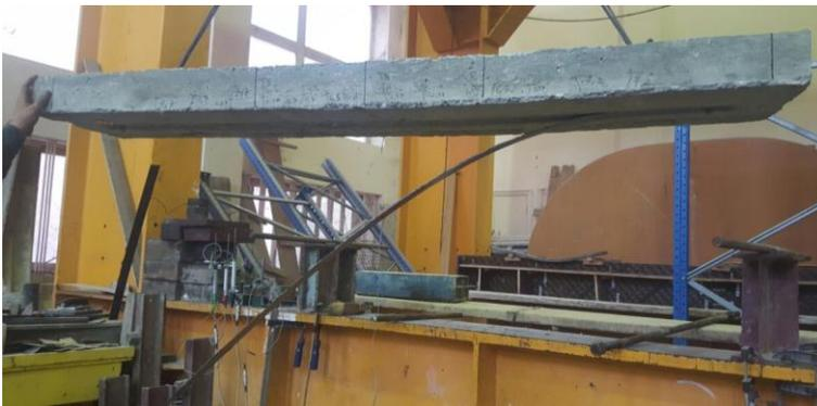
Figure 2. Bearing failure of the FRP Strip.
