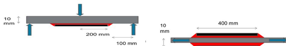
Figure 4. Scheme of the flexure test and the double strap test (from left to right)
