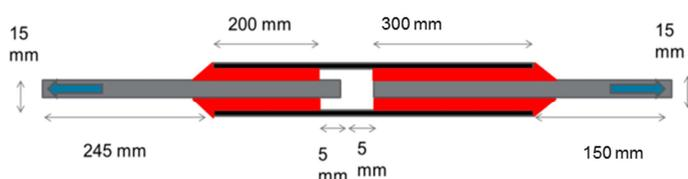
Figure 3. Scheme of the double lap shear test
