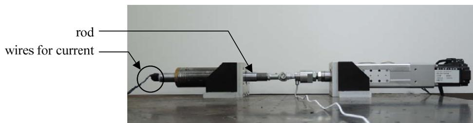
Figure 4. The experimental rig of the 400 N MR damper.
