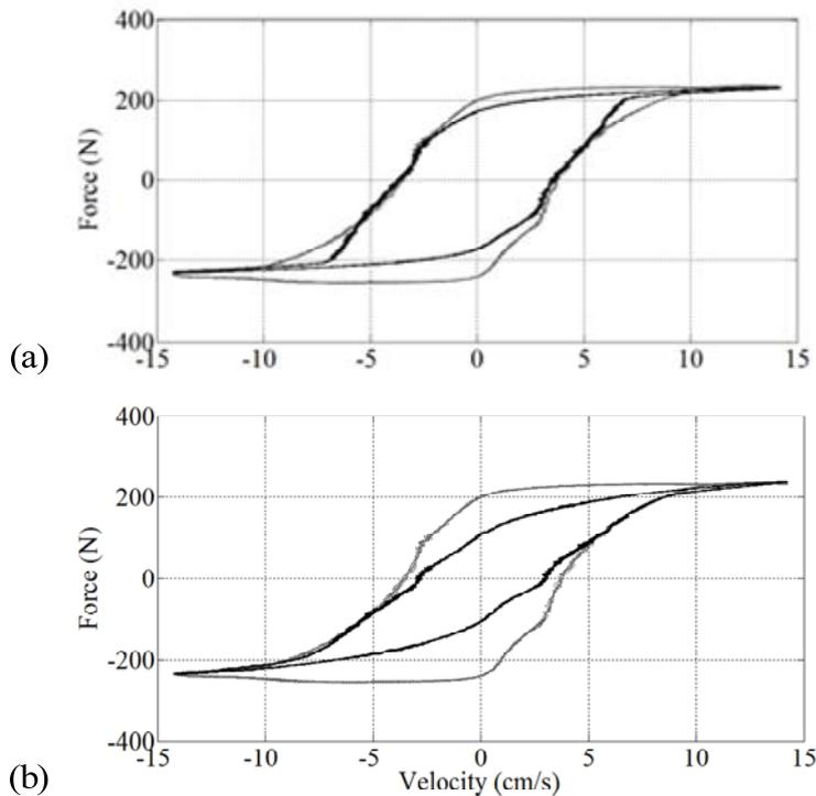
Figure 5. Comparison of parameter identification with sinusoidal excitations: (a) parameters selected to fit the linear part, and (b) parameters selected to fit the transition point.
