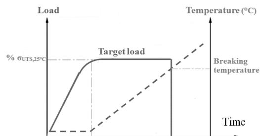
Figure 3. Transient-state (TS) path.
