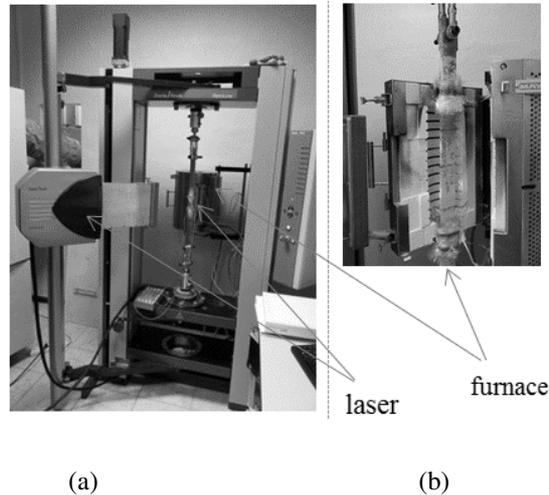
Figure 1. (a) The machine Zwick 20kN-furnace; (b) Furnace and specimen installed for a thermomechanical tensile test.
