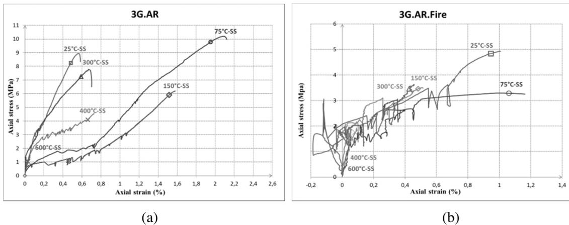
Figure 4. Behaviour of (a) 3G.AR and (b) 3G.AR.Fire in Steady-State (SS) tests.
