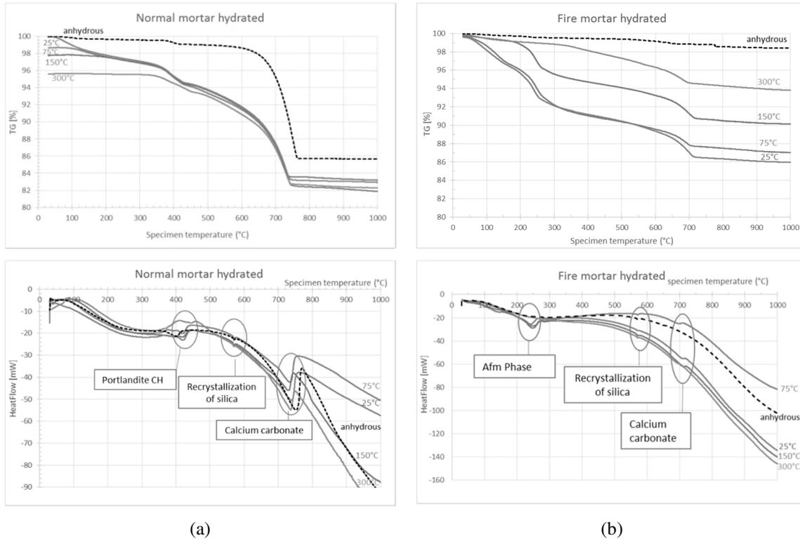
Figure 8. Thermogravimetric (TG) results of (a) the preheated-cooled normal mortar (of 3G.AR) and (b) of the preheated-cooled fire mortar (of 3G.AR.Fire); TG tests carried out on mortar samples that were previously preheated at different levels of temperature and cooled up to ambient temperature.
