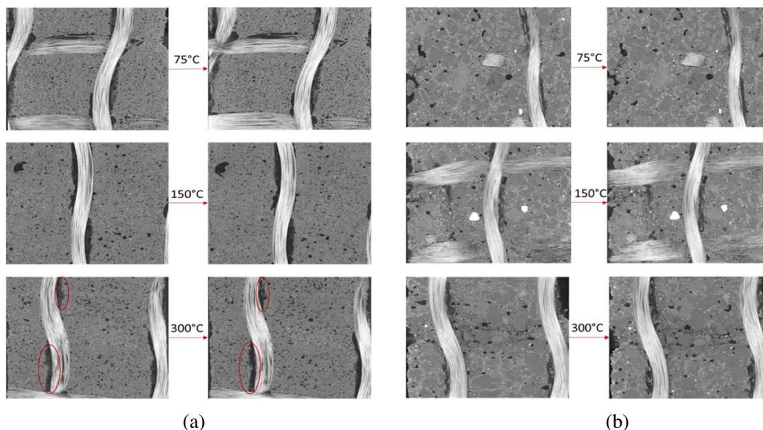
Figure 7. Raw images of (a) 3G.AR and (b) 3G.AR.Fire at 75°C, 150°C and 300°C
