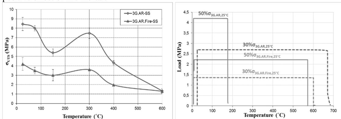
Figure 5. Average ultimate tensile strength ( $\sigma_{UTS}$ ) of 3G.AR and 3G.AR.Fire as a function of the temperature.
