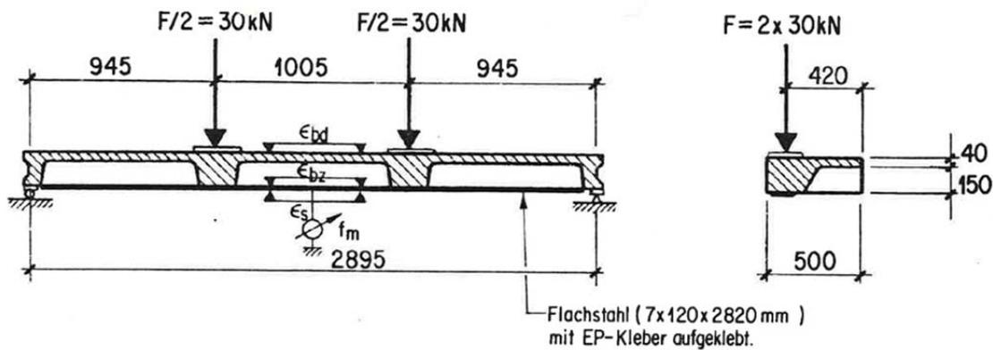
Figure 3: Dimension and measurements of the long-term test.
