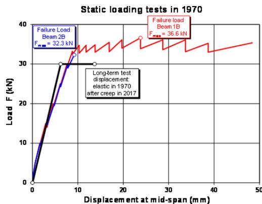
Figure 5: Load-displacement diagram of the static loading tests.
