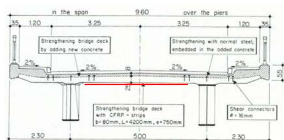
Figure 10: Cross-section of the bridge. Figure taken from Walser et al. (1997). The location of the CFRP strips are indicated with a red line.
