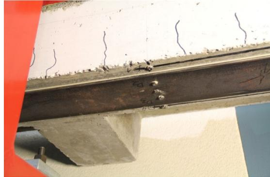
Figure 6: Failure mode in the static loading test on Beam 2B. Photo from the year 1970.
