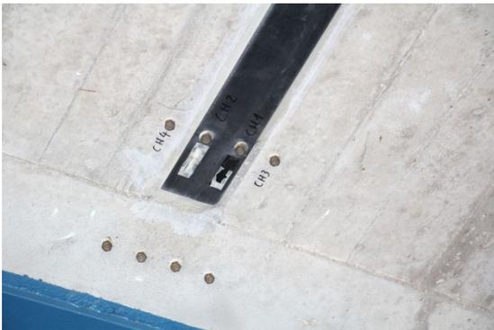
Figure 13: Measurement points at the end of a CFRP strip.
