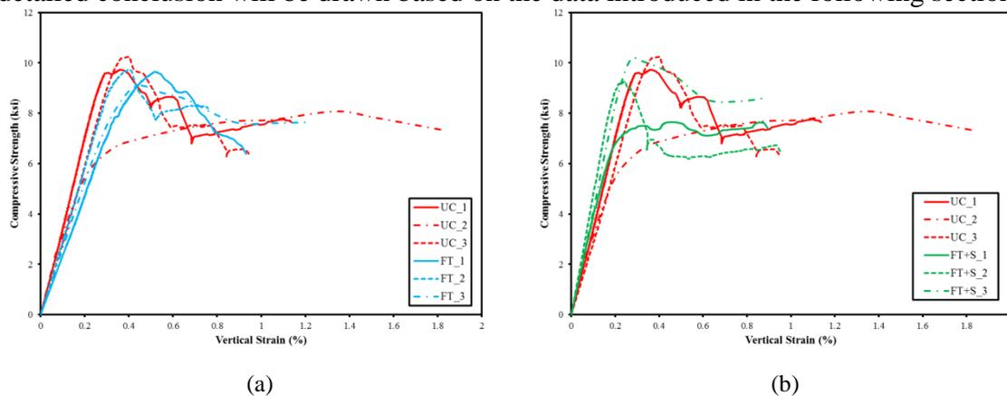
Figure 6. Stress-strain curves in vertical direction for: (a) UC vs. FT; (b) UC vs. FT+S.
