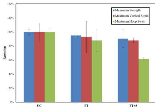
Figure. 7. Retention for maximum strength and strain of HC-FCS cylinders with  $\pm$  one standard deviation
