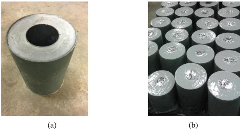
Figure 1. Specimen preparation: (a) HC-FCS cylinder; (b) epoxy coating on concrete surfaces
