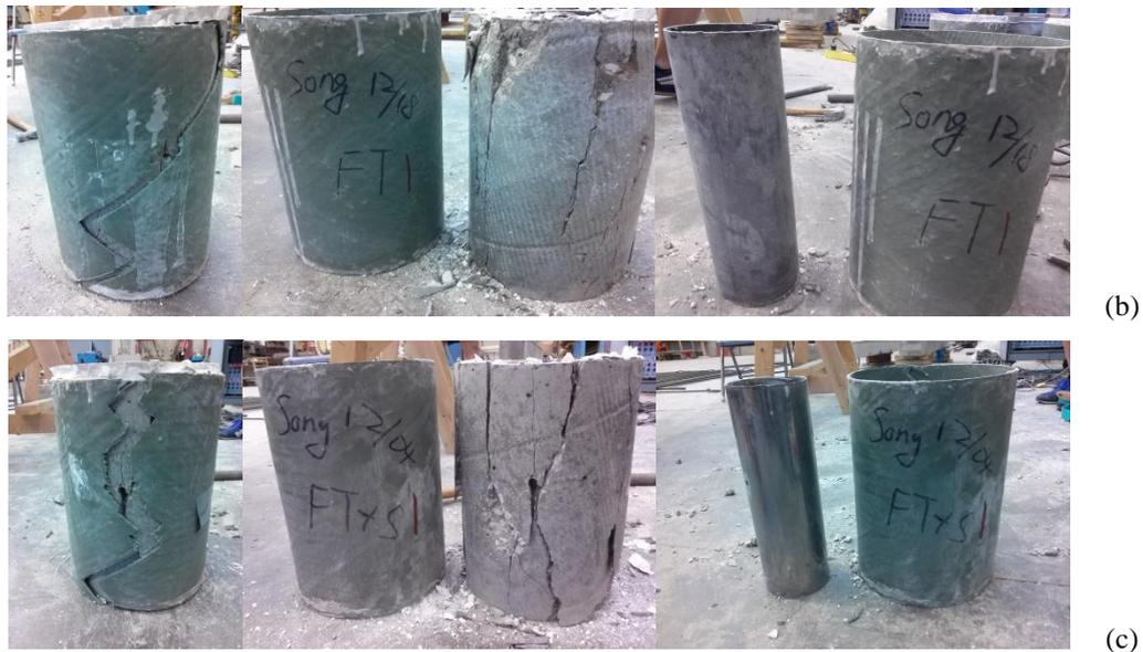
Figure 5. Failure modes of selected HC-FSC cylinders: (a) UC\_1; (b) FT\_1; (c) FT+S\_1
