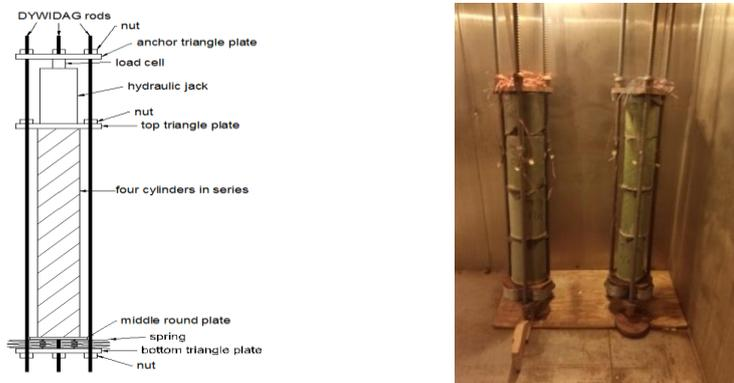
Figure. 2. Loading setup for environmental chamber
