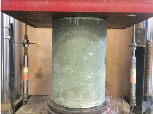
Figure. 4. Setup for the compression test on HC-FCS cylinders
