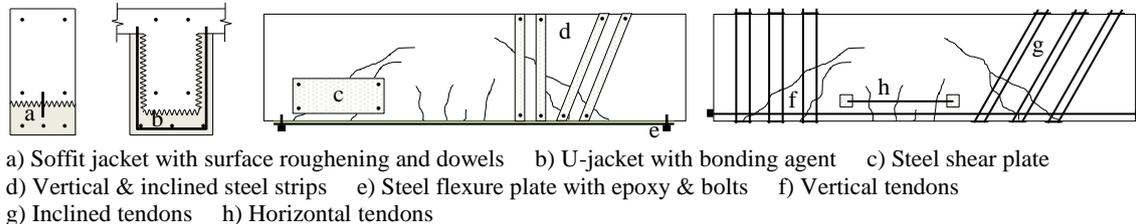
Figure 1. Retrofit methods considered: concrete jacketing, external steel elements, and external post-tensioning
