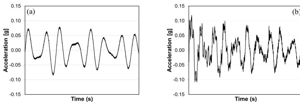
Figure 1. Acceleration signals at two locations on same structure: (a) slightly damaged; (b) severely damaged.
