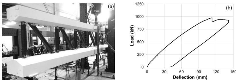
Figure 2. (a) Test setup and (b) load-deflection behaviour of the eight-panel truss girder.
