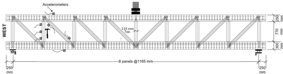
Figure 3. Dimensions and reinforcing details of the girder, and typical arrangement of accelerometers.
