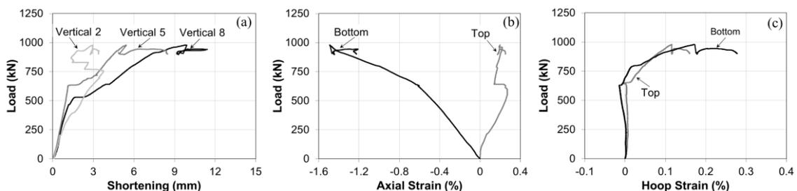
Figure 7. (a) shortening in the most stressed vertical elements; (b) axial strain and (c) hoop strain in the FRP tube of Vertical 8 during the static loading test.
