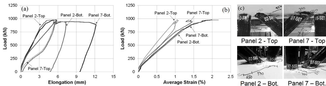
Figure 6. (a) elongation and (b) average strain in headed bars during the static loading test; and (c) state of damage after the test in the most stressed connections.
