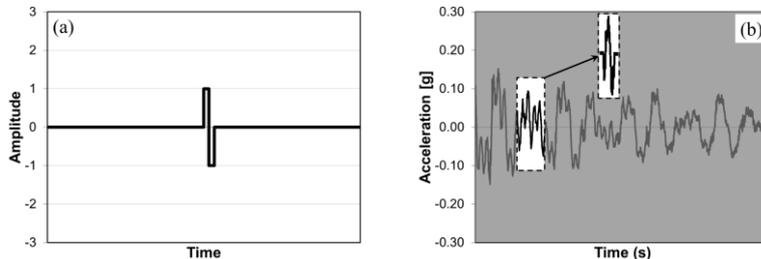
Figure 4. Similarity of (a) Haar wavelet and (b) damage-induced disturbances in a signal.
