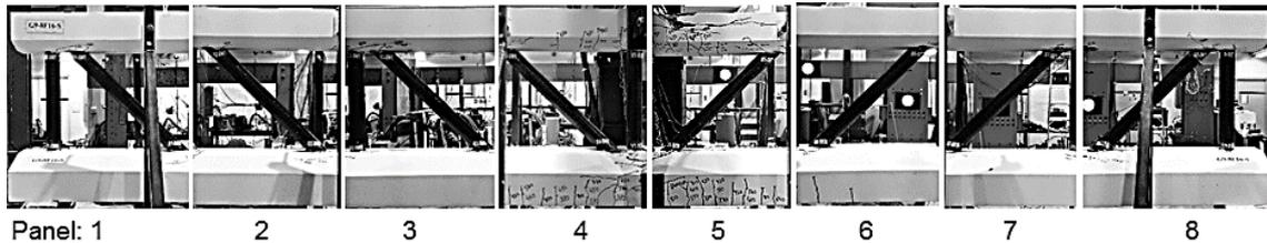
Figure 5. Structural condition of the concrete chords after performing the static loading test.
