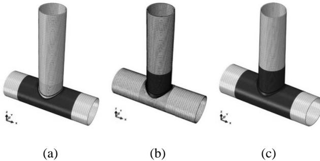
Figure 2. A typical FRP wrapped T-joint: a) Chord strengthening; b) Brace strengthening; c) Chord and brace strengthening
