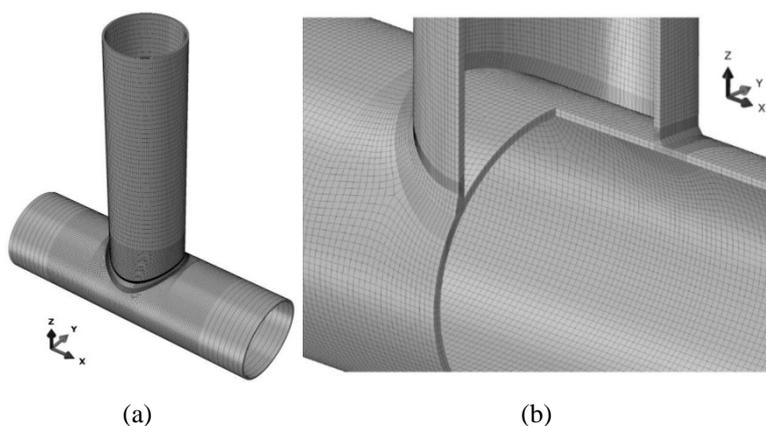
Figure 1. The mesh generated for the T-joint (JISSP joint 1.13) using the sub-zone method: a) Isometric view; b) Mesh enlargement
