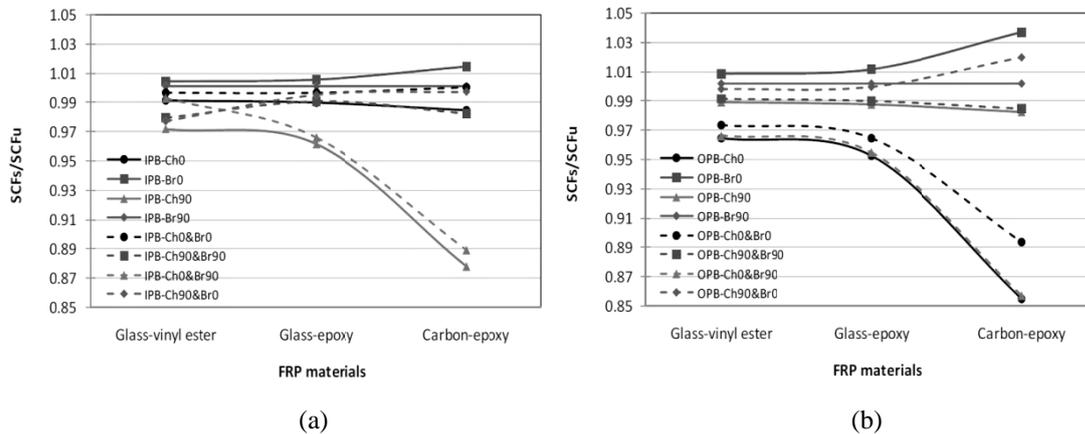
Figure 4. Ratio of SCF distribution in FRP strengthened tubular T-joint with different FRP materials to SCF distribution in un-strengthened joint: a) In-plane bending moment; b) Out-of-plane bending moment
