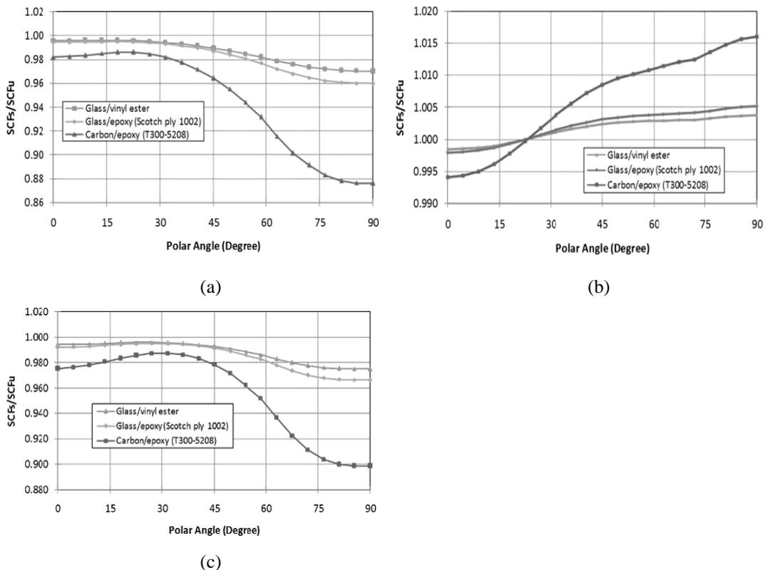
Figure 3. Ratio of SCF distribution in FRP strengthened tubular T-joint with different FRP materials to SCF distribution in un-strengthened joint: a) Chord member is strengthened; b) Brace member is strengthened; c) Both chord and brace are strengthened
