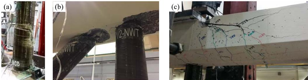
Figure 10. (a) Rupture of the vertical GFRP tube; (b) Fracture of the diagonal headed bars; (c) Crushing of concrete in the top chord
