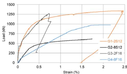
Figure 7. Load vs. maximum strain in headed bars.
