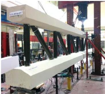
Figure 5. Test setup of the 8-panel girder.
