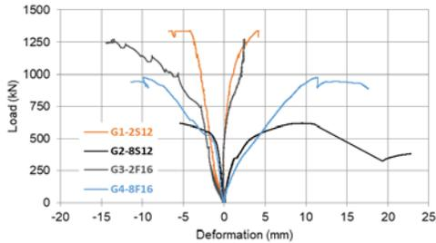
Figure 8. Deformations of the truss members
