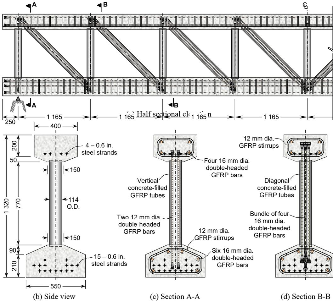
Figure 2. Dimensions and reinforcing details of the FRP-reinforced 8-panel girder.
