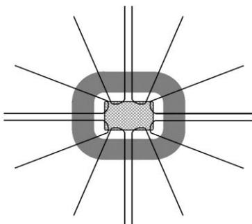
Figure 4. Cross-hatched area shows the region where the shear reinforcement can be considered.
