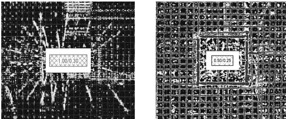
Figure 2. Radar images of punching shear reinforcement systems (left: Riss-Stern, right: steel shear head, generated from several image scans [recontec.ch (2016)]).
