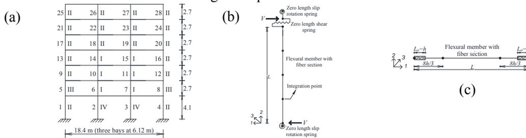
Figure 1. a) Geometric configuration of the transverse, b) columns, and c) beams models.
