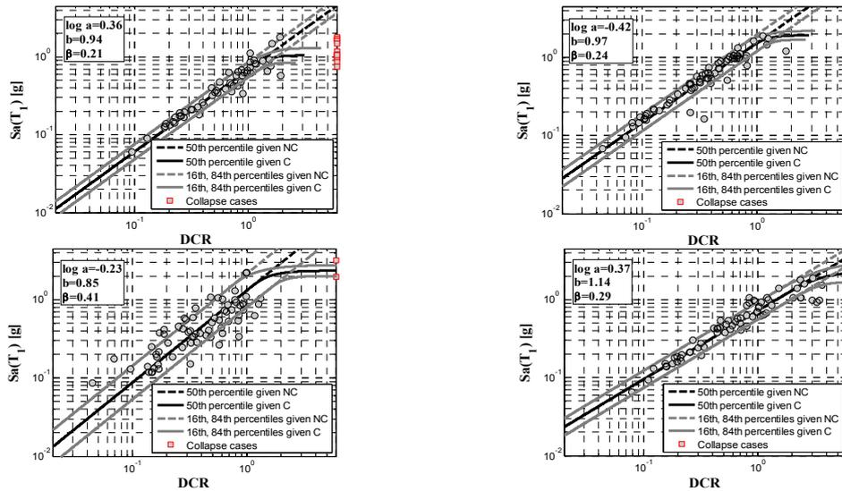
Figure 3 Cloud regression for LS<sub>PL</sub>: a) bare frame, b) RC jacketing, c) shear wall and d) FRP wrapping.
