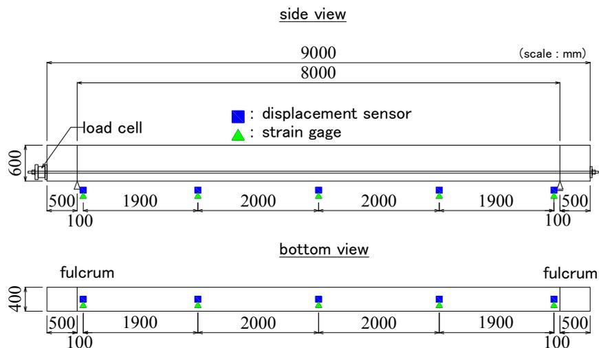
Figure 4. Position of measuring apparatus
