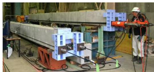
Figure 3. Installing fail-safe reinforcement cable
