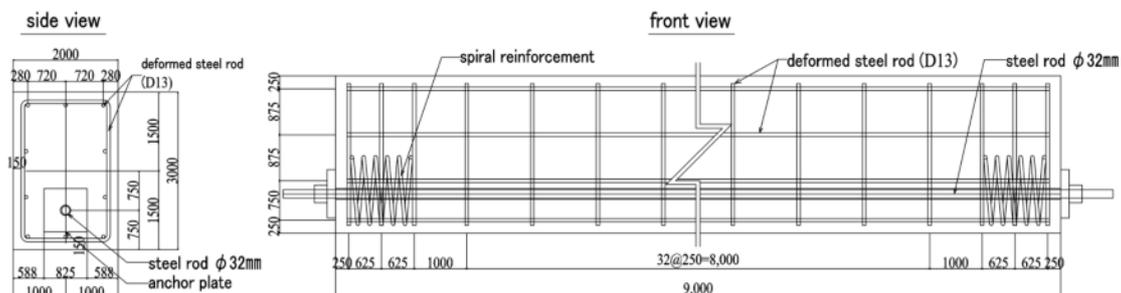
Figure 1. Details of PC girder
