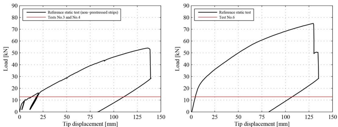
Figure 6. Load level: (Left) Strengthened slabs with non-prestressed strips and mastic asphalt (Slabs No.3 and No.4); (Right) Strengthened slab with prestressed strips and without mastic asphalt (Slab No.6).
