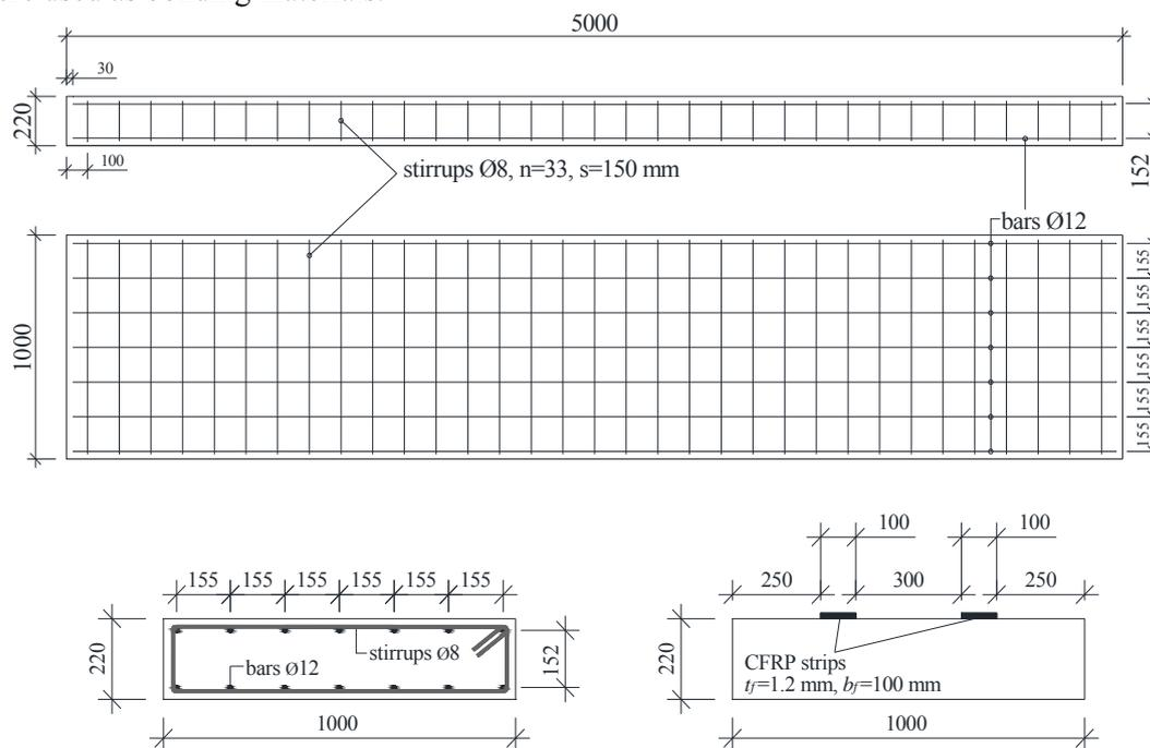
Figure 2. Geometry of the slabs and distribution of the steel reinforcement.
