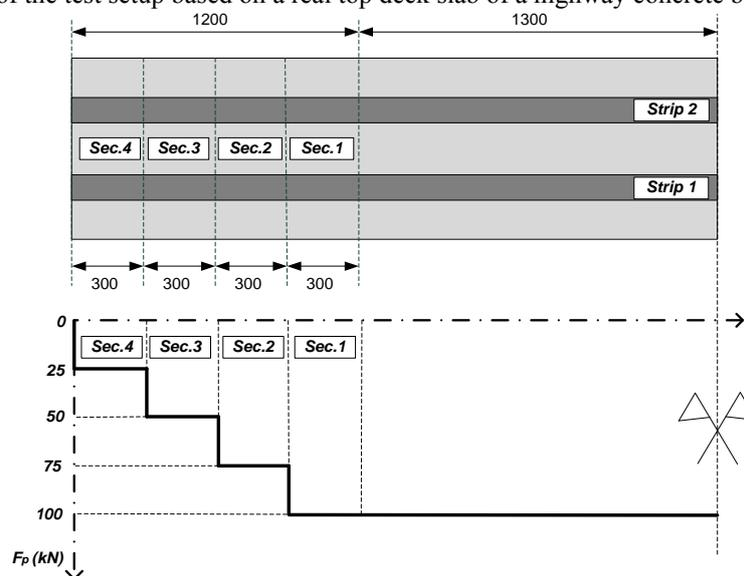
Figure 4. Distribution of the prestress force in each strip after releasing.
