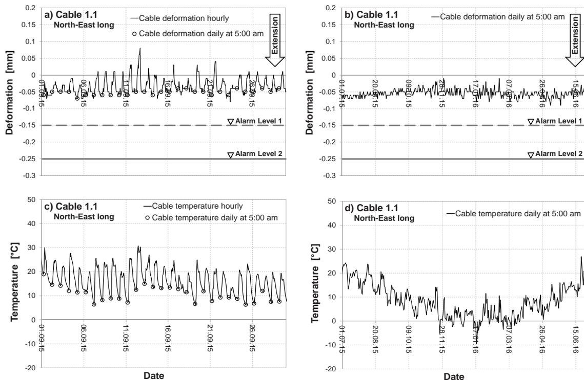
Figure 6. Deformations of cable 1.1: (a) comparison of hourly variability vs. daily measurements at 5:00 am; (b) development of 5:00 am measurements during 12 months; and (c), (d) corresponding cable temperatures.
