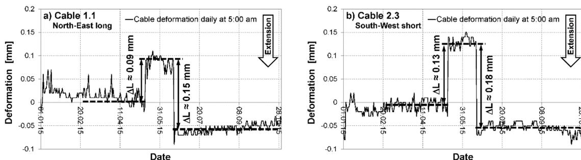
Figure 7. Deformations of (a) long and (b) short cable during cutting and re-application of pavement.
