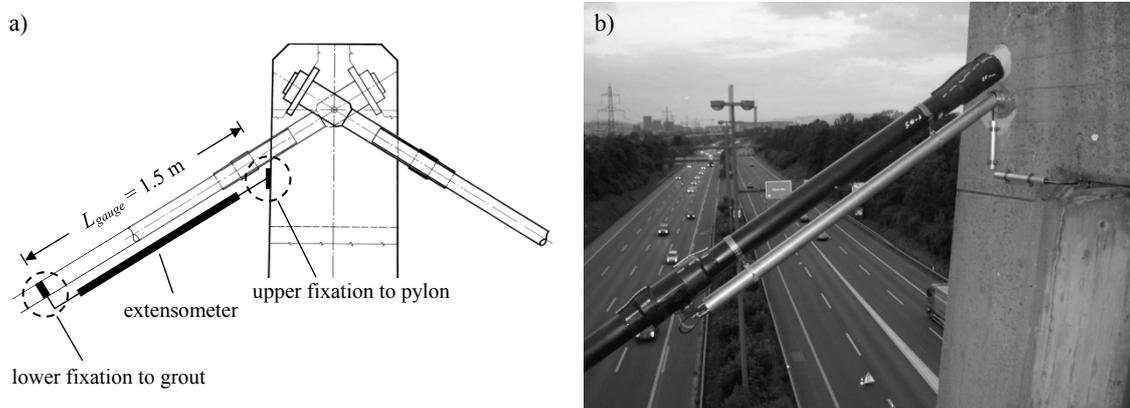
Figure 5. Fixation of extensometer: (a) schematic sketch and (b) photo of implemented solution.
