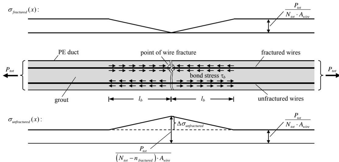
Figure 3. Cable stress distribution in the vicinity of local wire fractures; bond related interaction between fractured and unfractured wires.
