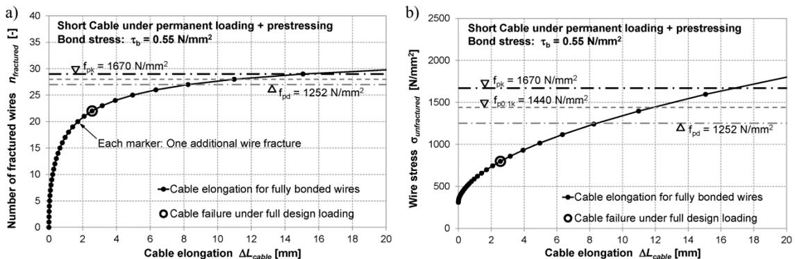
Figure 4. Cable elongation due to wire fractures: (a) relationship between number of fractured wires and elongation, (b) relationship between stress in unfractured wires and cable elongation.
