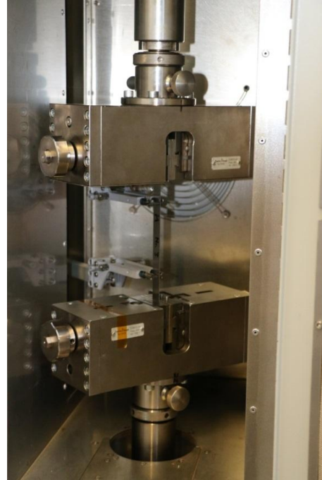
Figure 4. A 20 kN Zwick machine equipped with a climate chamber. The machine was used for prestraining and activation of the Fe-SMA samples.
