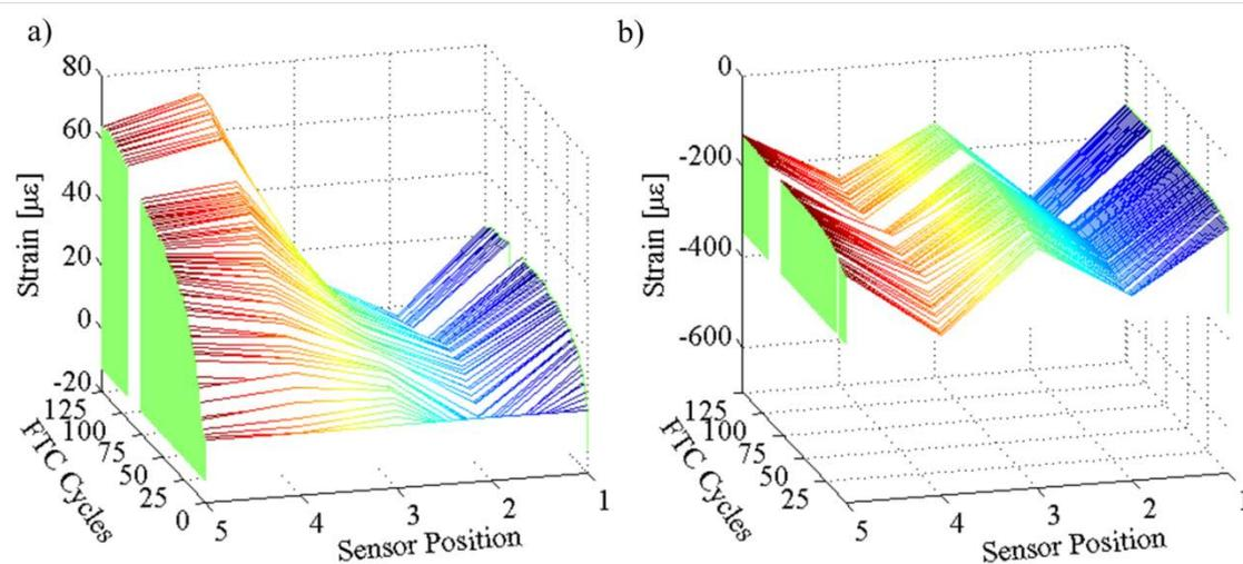
Figure 8: Maximum (a) and minimum (b) strains observed during FTC.
