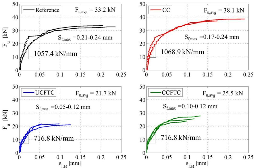
Figure 6: Force-slip relationship for every lap-shear test.
