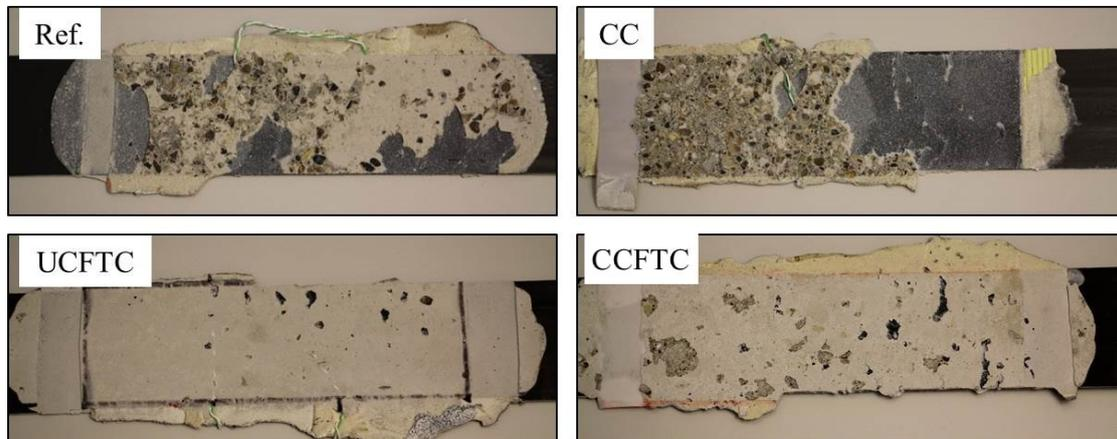
Figure 7: Typical failure surface for every exposure case.
