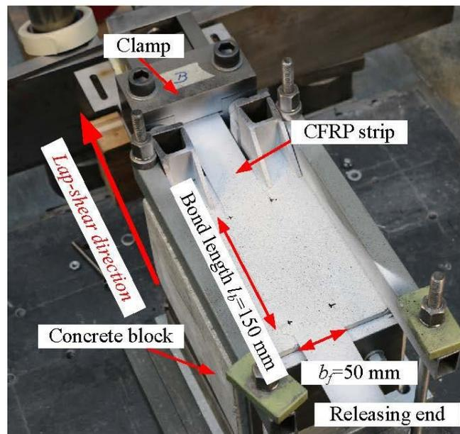
Figure 3: Concrete block with prestressed CFRP anchored with a single section gradient anchorage and painted with a speckle pattern for 3D-DIC measurements.
