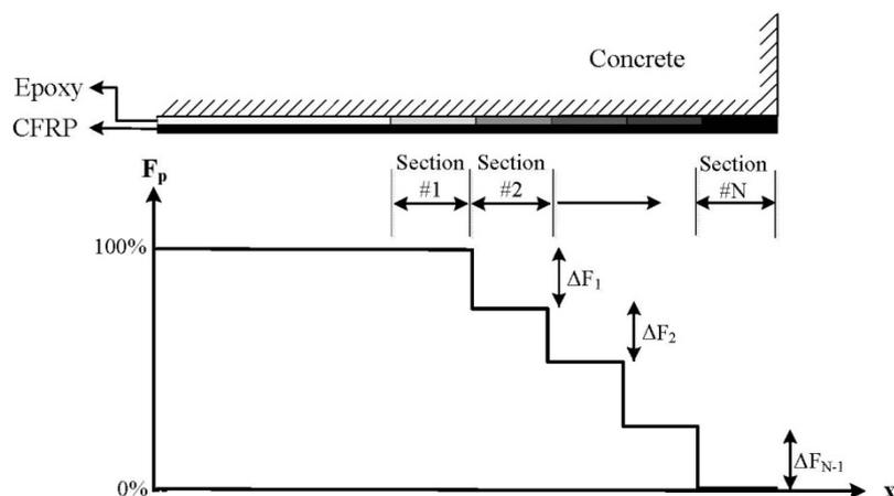
Figure 1: Schematic description of the gradient anchorage.
