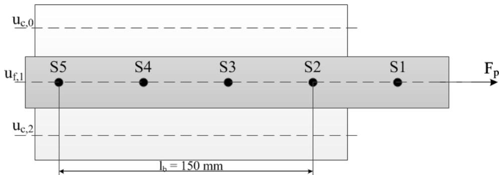
Figure 5: Top view of specimens, with markers denoting FOS locations and sections for 3D-DIC
