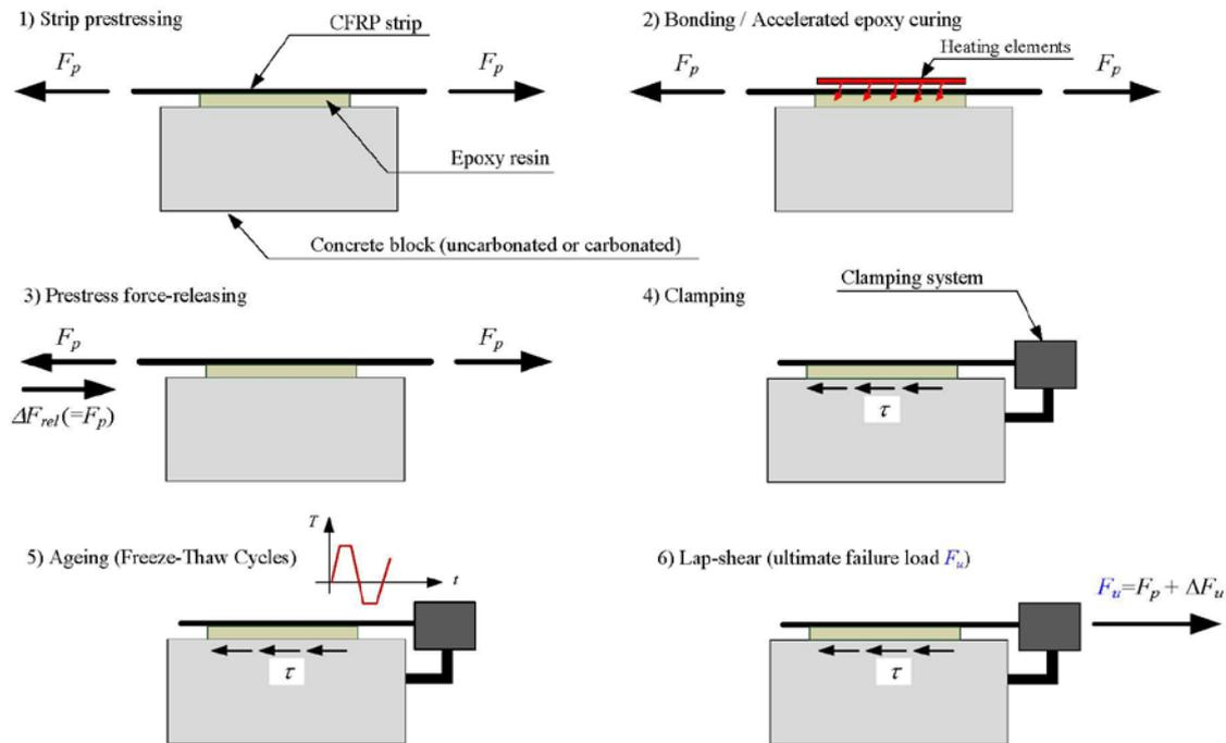
Figure 2: Schematic overview of the experimental procedure.
