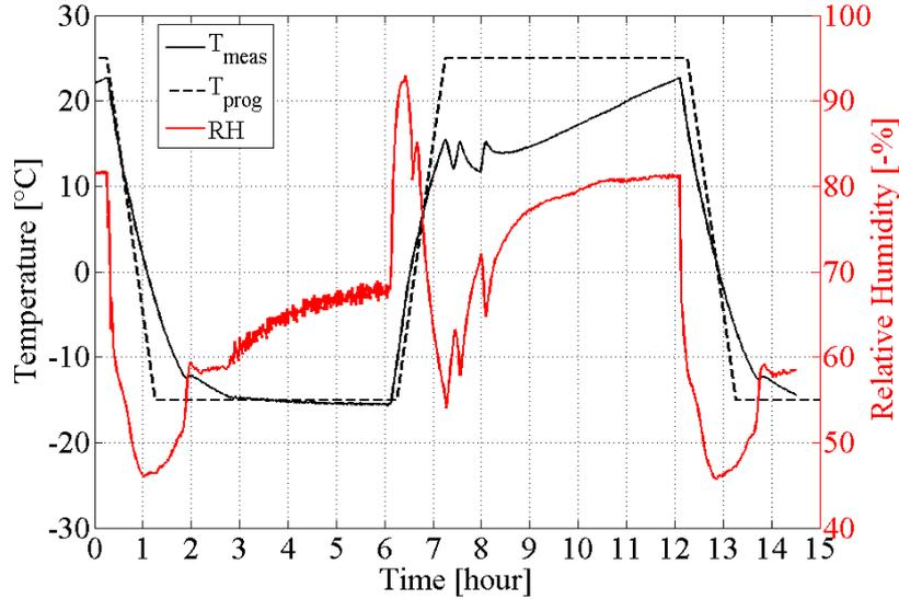
Figure 4: Programmed temperature curve and measured temperatures and RH during a single FTC.
