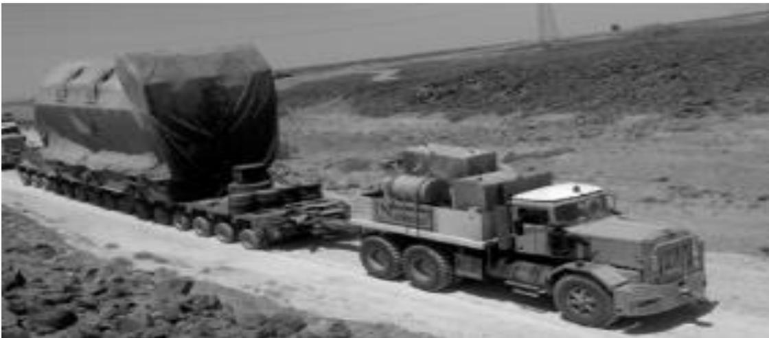
Plate 2. 277 000 kg superload on single lane Goldhofer hydraulic trailer.
