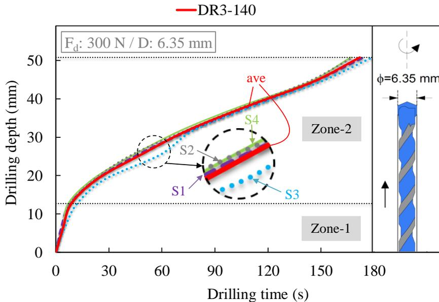
Figure 2. Drilling depth vs. drilling time curves for DRT3 mortars.
