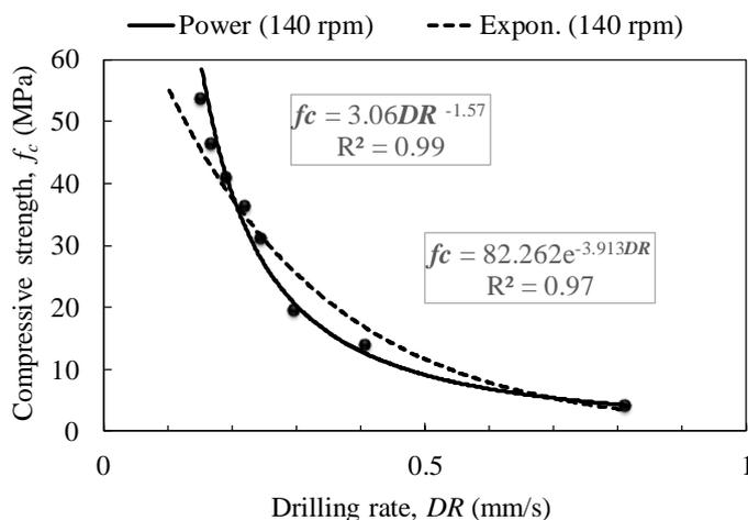
Figure 3. Relationship between the compressive strength and the drilling rate of the mortars.
