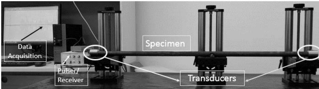
Figure 4 Experimental setup for contact type PZT based Ultrasonic system
