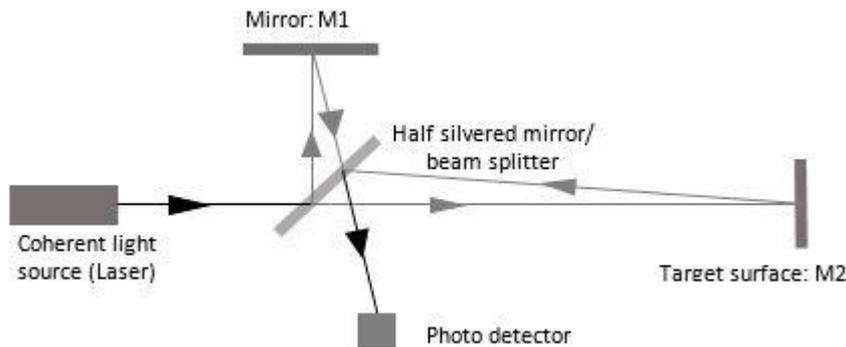
Figure 1 Working principle of Interferometer
