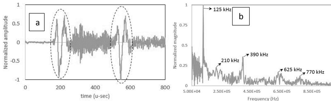
Figure 5 Signal acquired using non-contact technique (a) Time series data and (b) Frequency data
