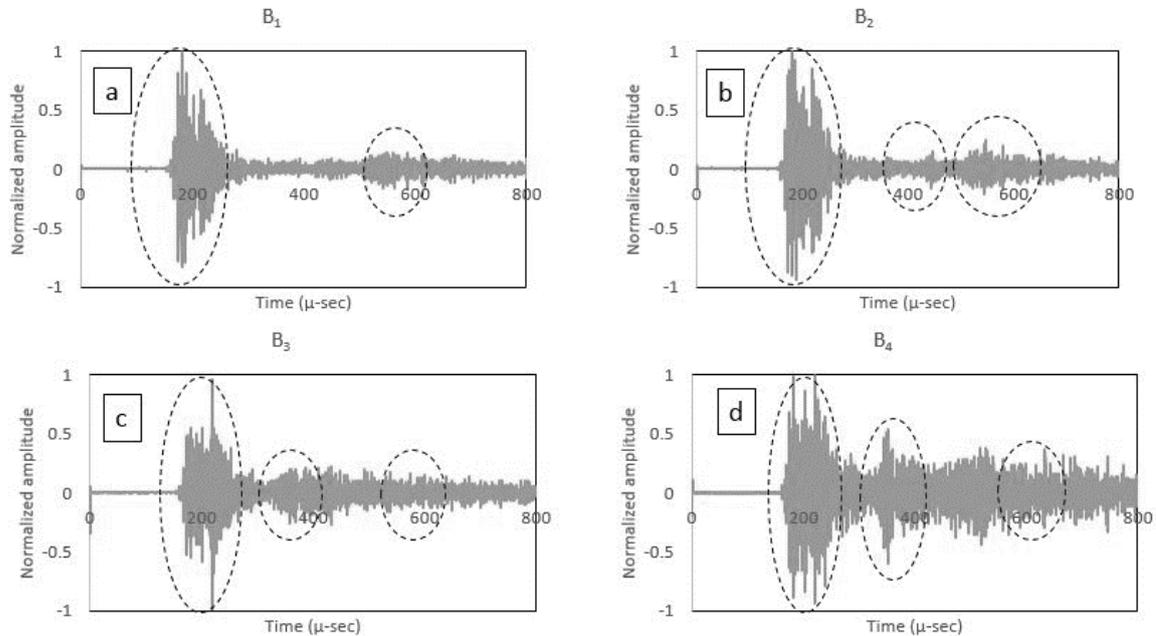
Figure 8 Time series data acquired using contact type monitoring technique (1MHz transducers) with different percentages of reduction in cross section area
