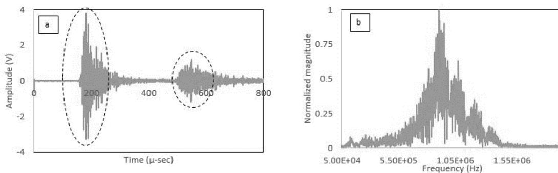
Figure 7 Signal acquired using contact based PZT system of 1MHz transducers (a) Time series data and (b) Frequency data
