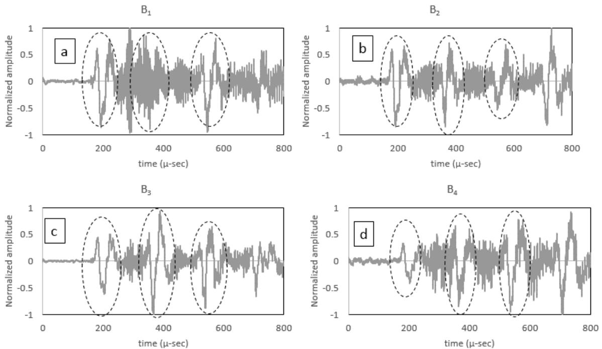
Figure 6 Time series data acquired using non-contact monitoring technique with different percentages of reduction in cross section area
