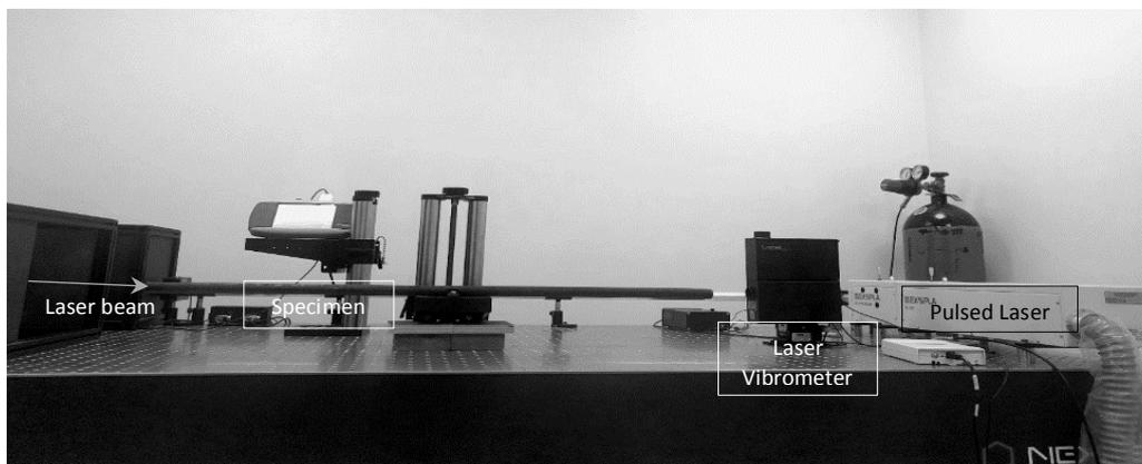
Figure 2 Experimental setup for Non-contact type Laser Ultrasonic system
