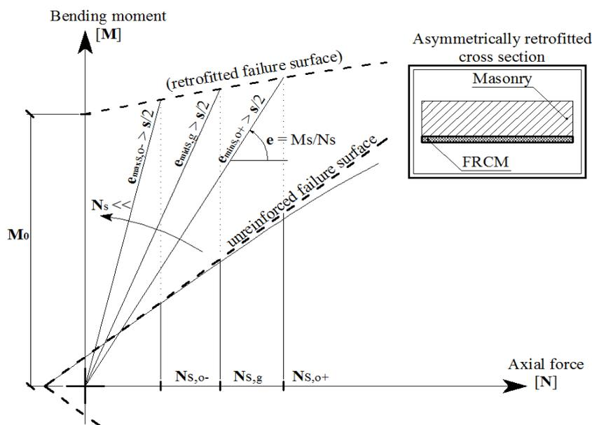
Figure 3. FRCM retrofit effect on the thrust line eccentricity  $e$ .
