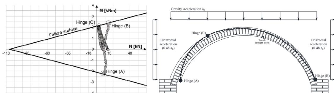
Figure 4. Unreinforced vault: thrust line and NM points at 0.48g load condition on failure surface.
