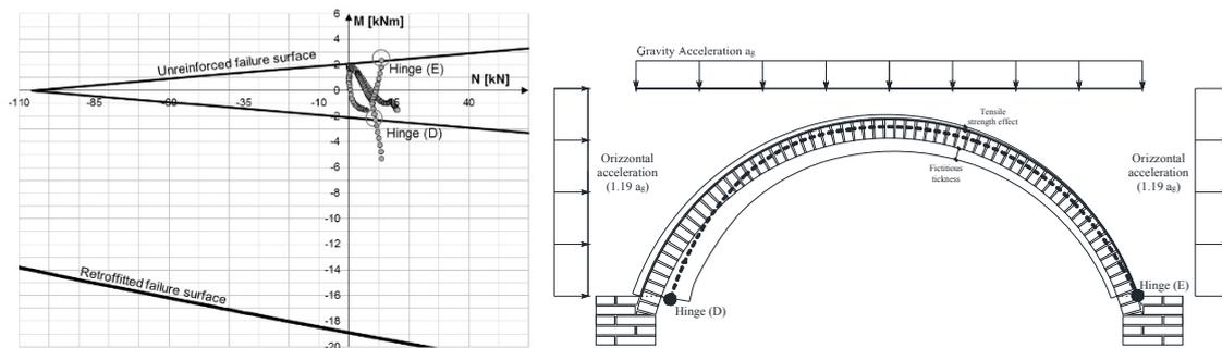
Figure 5 Reinforced vault: thrust line and NM points at 1.19g load condition on failure surface.
