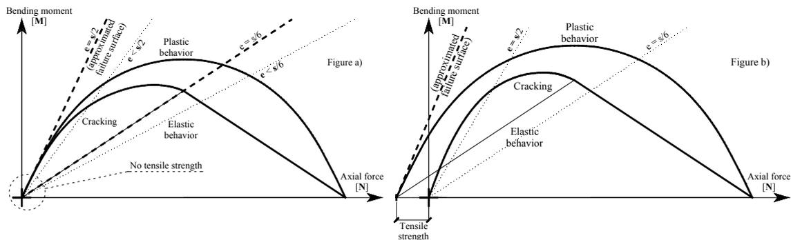
Figure 1. Unreinforced vault: bending moment-axial force failure surface with and without tensile strength.
