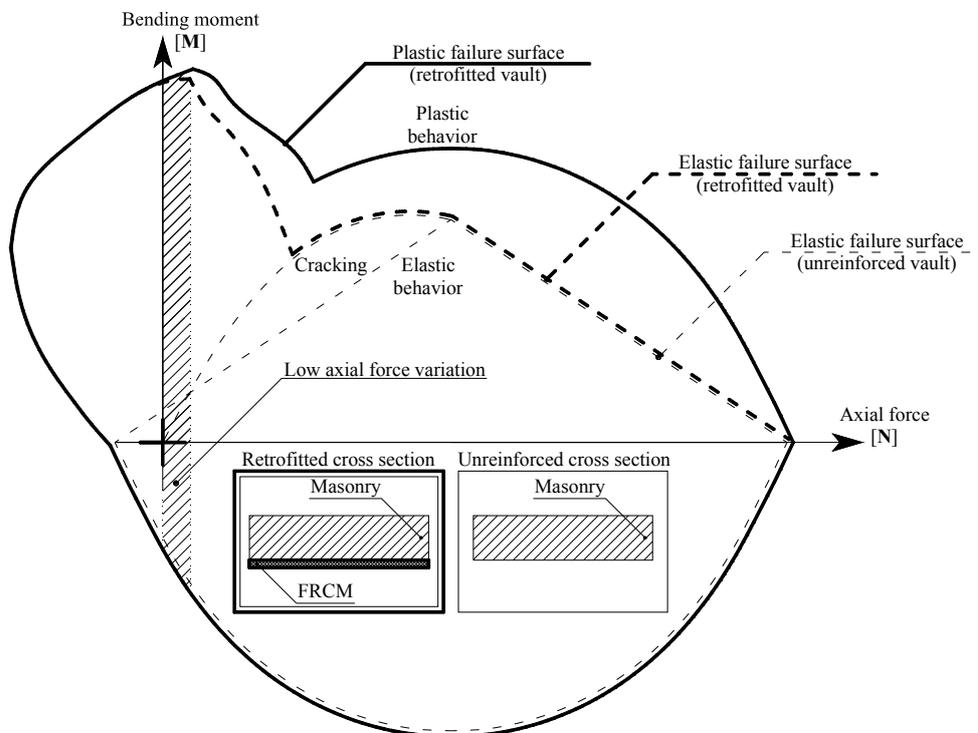
Figure 2. Retrofitted vault: bending moment-axial force failure surface.
