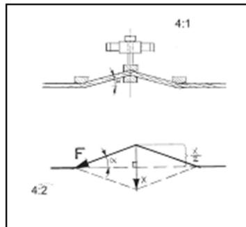
The resultant force affects the pull rod which is firmly connected with the flat centre support. The pull rod affects in its turn the load cell, which gives an electrical signal which is proportional to the force. The signal is amplified, converted and indicated on the LCD display of the instrument.
