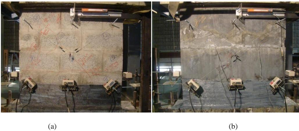
Fig. 3: Cracking Pattern in (a) NCMW and (b) NCMWR
