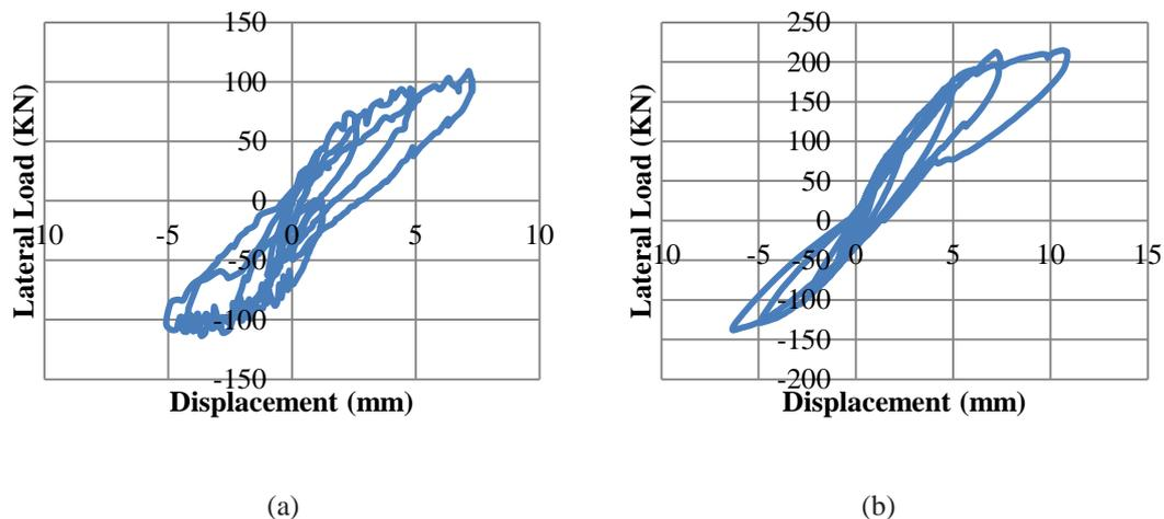
Fig. 4: Load-Displacement Hysteresis (a) NCMW (b) NCMWR
