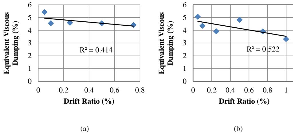
Fig. 5: Equivalent Viscous Damping (a) NCMW (b) NCMWR
