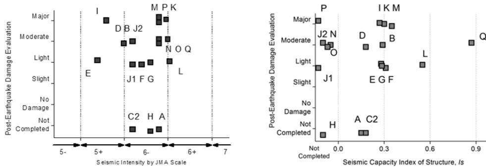
(a) with Seismic intensity. (b) with Seismic capacity index of structure,  $I_s$ .
