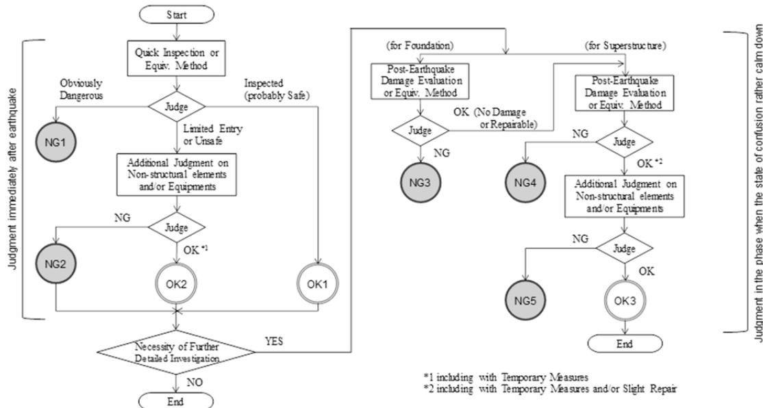
Figure 4. Flowchart of judgment on continuous use of damaged building.
