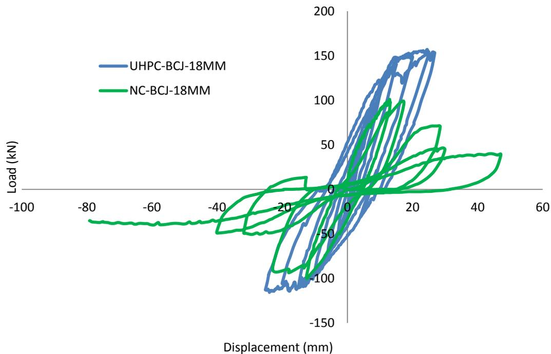
Fig. 6: Load vs displacement graph for specimen UHPC-BCJ-18MM & NC-BCJ-18MM
