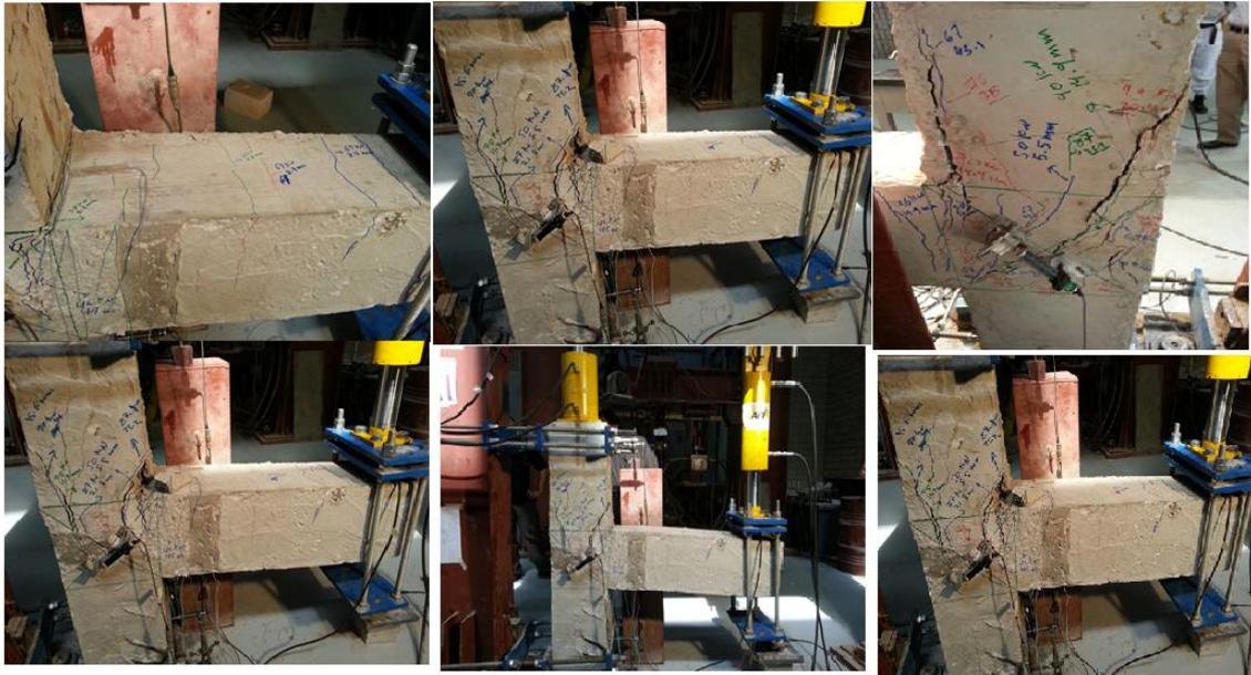
Fig. 4: Crack pattern for specimen NC-BCJ-18MM
