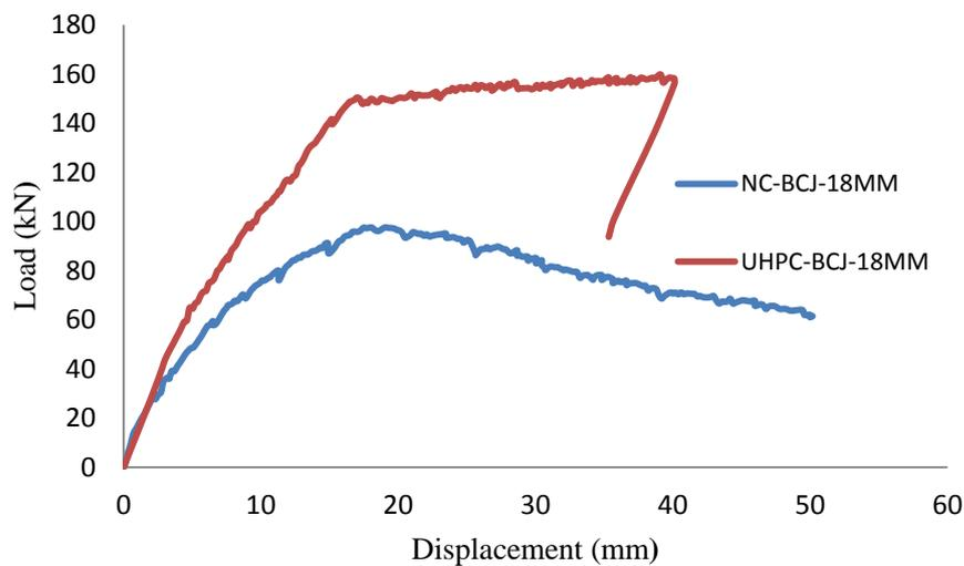
Fig. 3 Load vs. displacement for specimen UHPC-BCJ-18MM & NC-BCJ-18MM
