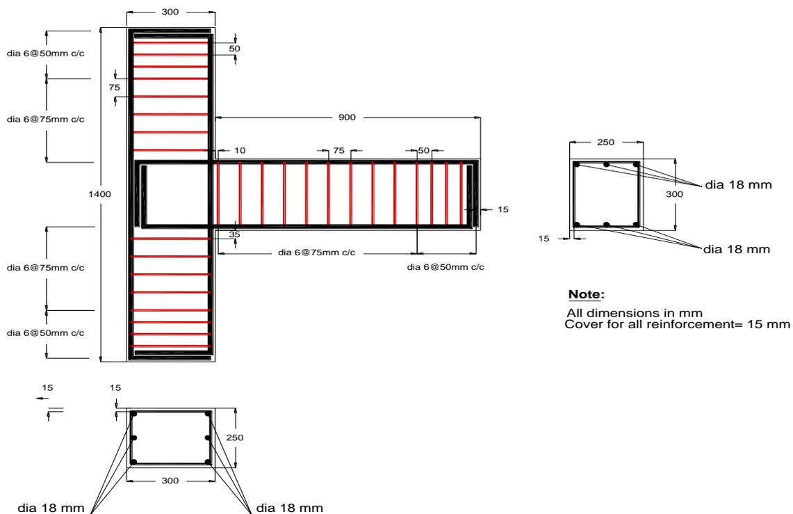
Fig. 1 Geometric and reinforcement details for BCJ-18 MM
