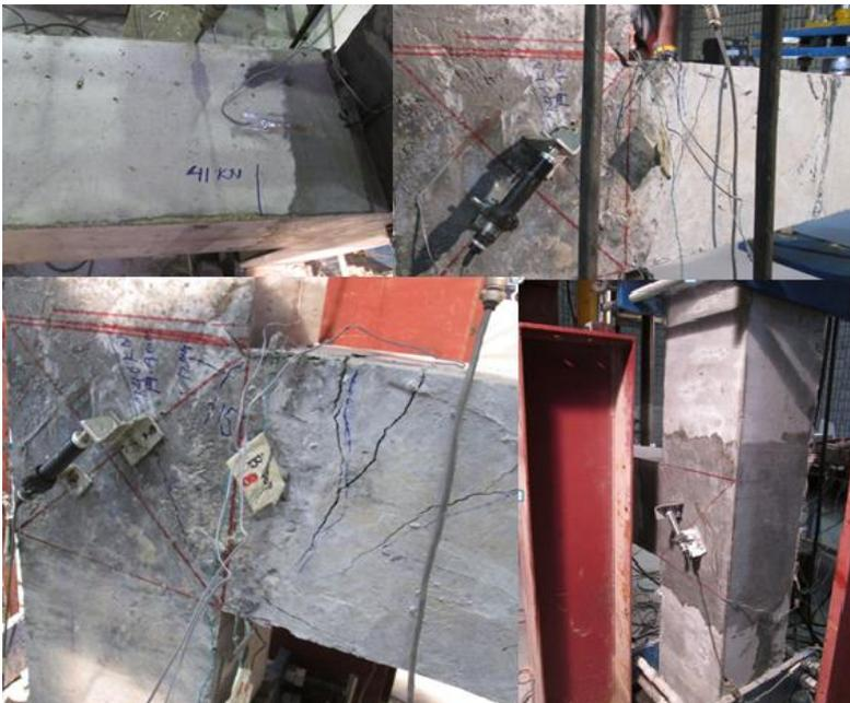
Fig. 5: Crack pattern for specimen UHPC-BCJ-18MM
