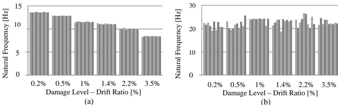
Figure 3. Identified natural frequencies at different damage levels using ERA based on impact hammer data for 10 different initial-end points (a) S1 (b) S2
