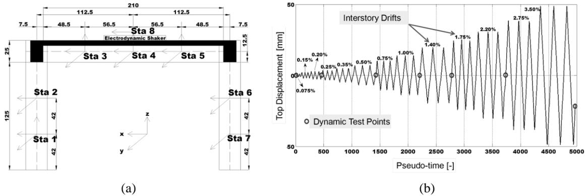
Figure 2. (a) Accelerometer layout, (b) sequence of static and dynamic tests.
