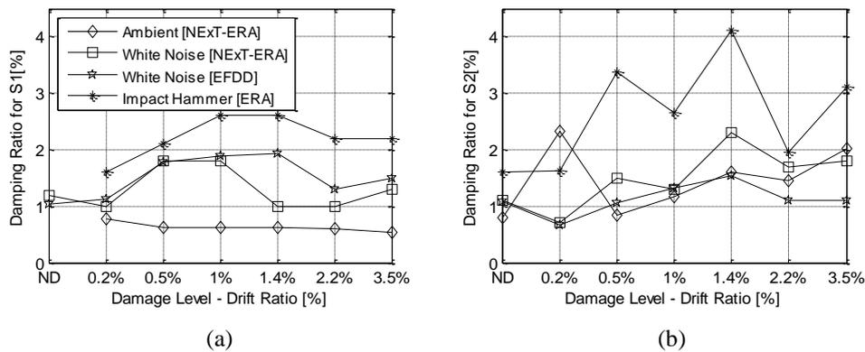
Figure 4. Damping ratio-damage level relationship with different methods (a) S1 (b) S2
