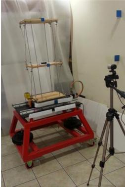
Figure 2. Test setup; Shaking Table, test structure and video recording system.
