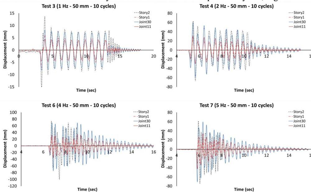
Figure 6. Dynamic test (high-amplitude) time-histories
