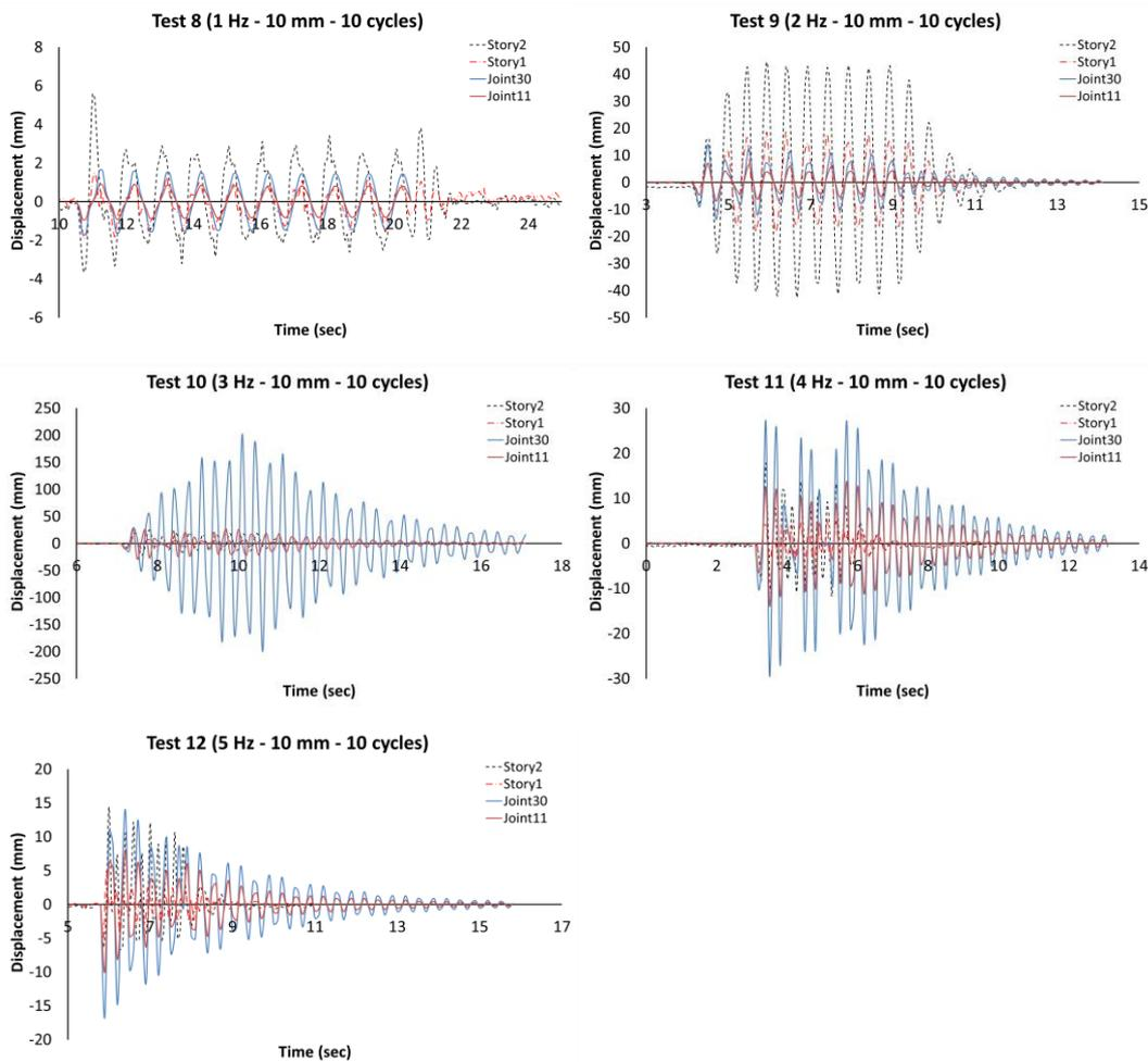
Figure 7. Dynamic test (low-amplitude) time-histories
