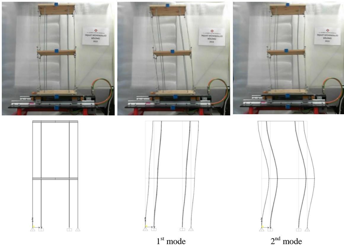
Figure 4. First two mode shape of the test structure and the numerical model.
