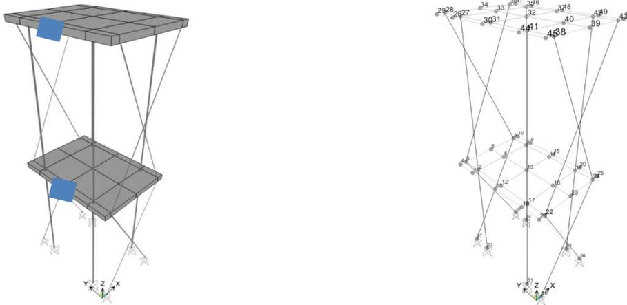
Figure 3. Numerical model of the test structure, markers and corresponding joints on FEM model.
