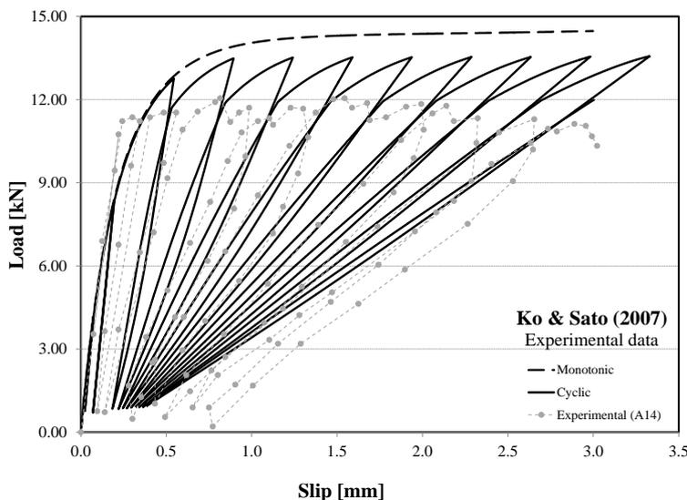
Figure 4. Load-slip response under monotonic and cyclic actions of FRP strips glued to concrete (Ko & Sato, 2007).
