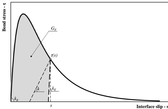
Figure 2. Fracture work spent as defined in eq. (8).
