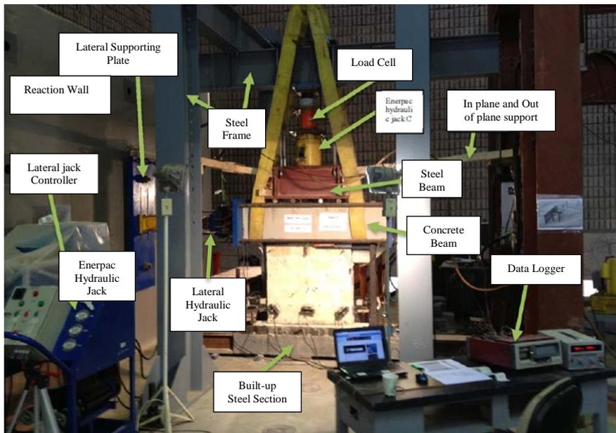
Figure 2. Cyclic Test Setup of Control wall
