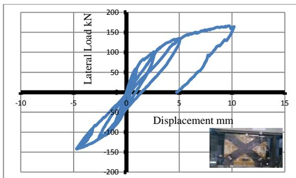
Figure 7. Lateral force-deformation hysteresis loop diagram for strengthened specimen
