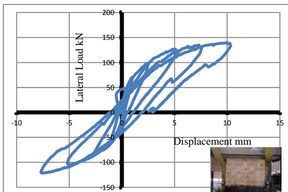
Figure 5. Lateral force-deformation hysteresis loop Diagram for Control specimen
