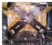
(a) Strengthening of Undamaged Wall
