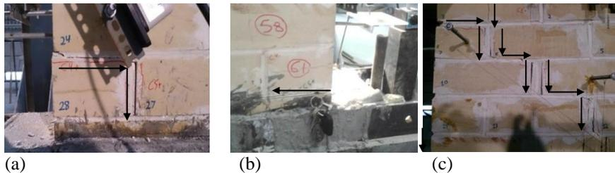
Figure 4. Cracking and failure mode of control specimen
