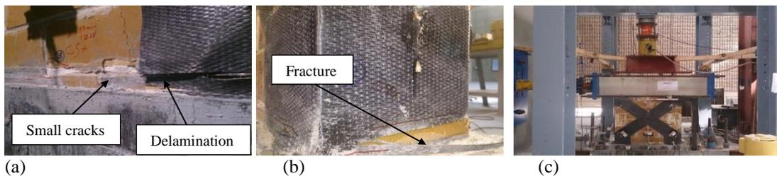
Figure 6. Some cracking patterns of undamaged specimen strengthened with CFRP
