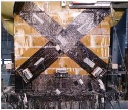
Figure 8. Cracking patterns of retrofitted specimen
