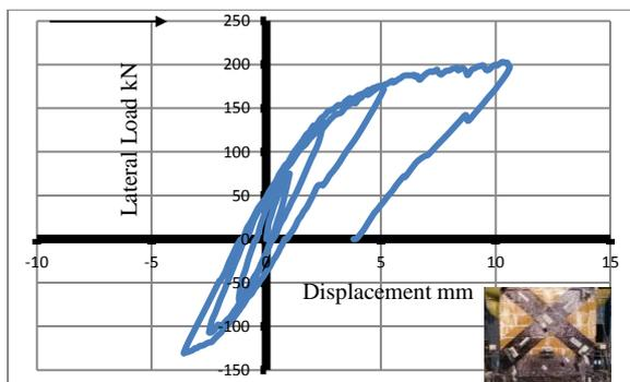
Figure 9. Lateral force-deformation hysteresis loop diagram for retrofitted specimen
