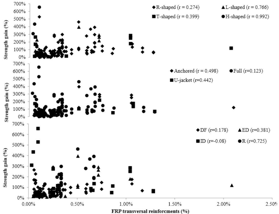
Figure 3. Strength gain versus FRP reinforcement ratio
