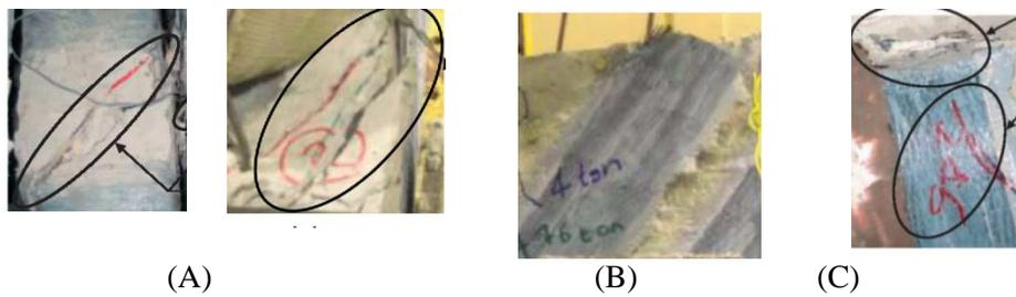
Figure 2. Various failure modes observed: A) DF, B) ED and C) ID.
