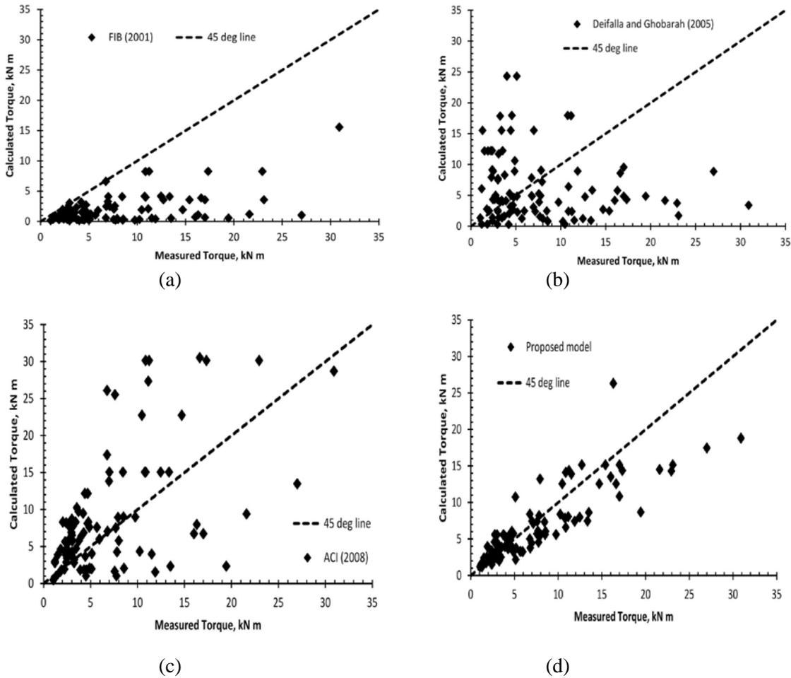
Figure 4 – Measured torque versus calculated using a) FIB (2001), b) Deifalla and Ghobarah (2005), c) ACI (2008), d) Proposed formula.
