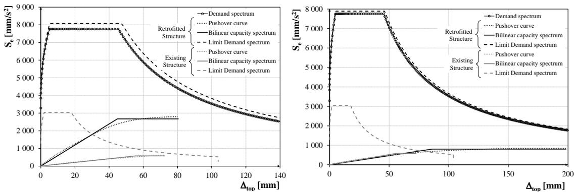
Figure 4. Seismic analysis of the retrofitted structure (solution N.1 on the left and N.3 on the right).
