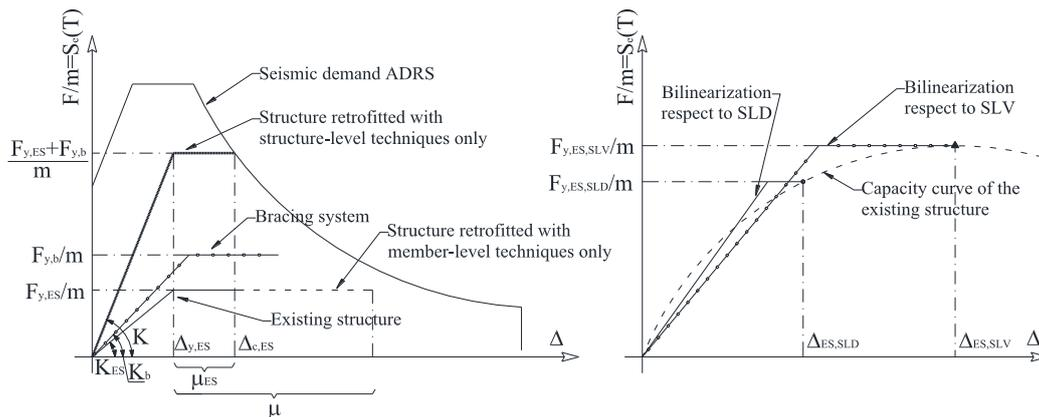
Figure 1. Idealised capacity curves for the structural systems involved in the rational retrofitting strategy.
