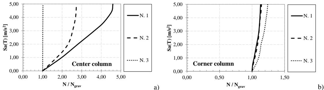
Figure 7. Maximum axial loads: a) central columns and b) corner column
