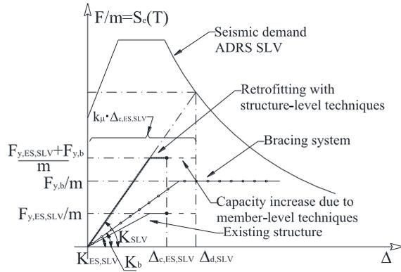
Figure 3. Retrofitting objective at SLV with required increase of capacity  $k_\mu$ .
