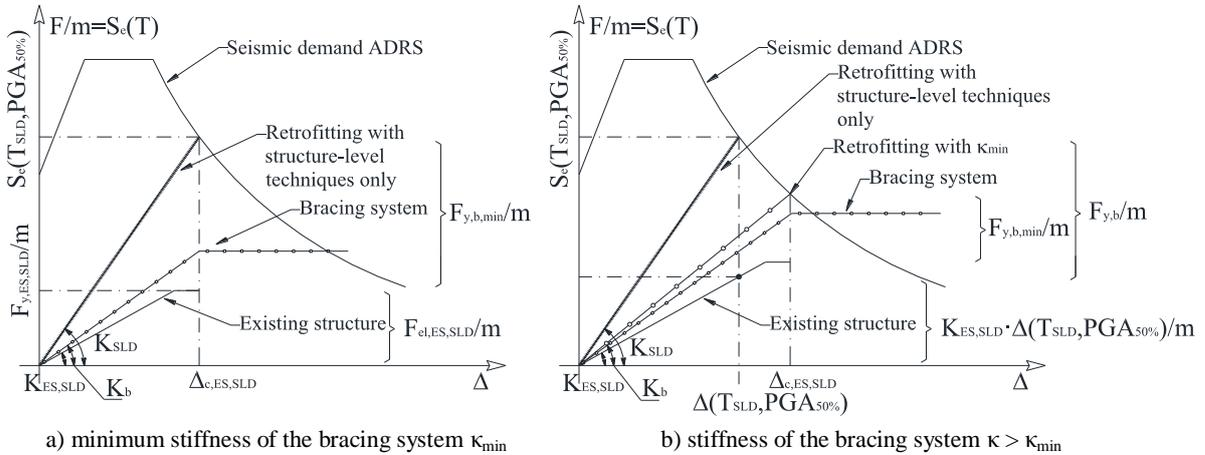
Figure 2. Retrofitting objective at SLD.
