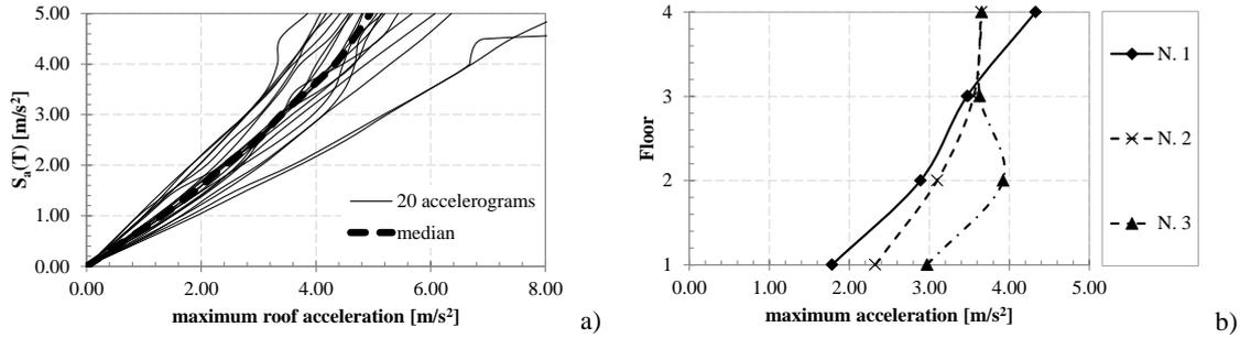
Figure 6. a) Maximum roof acceleration from IDA of the retrofitting solution N.1; b) Maximum floor accelerations of the three retrofitting solutions
