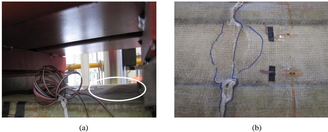
Figure 5. Failure modes: (a) outward skin wrinkling in the control panels, and (b) compression failure in the control and conditioned panels.
