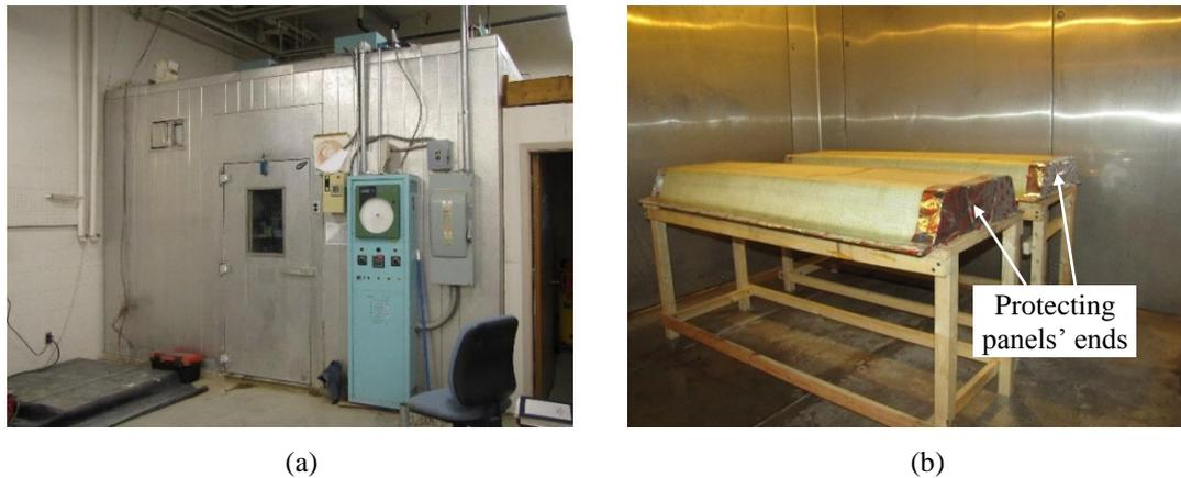
Figure 2. Thermal cycling: (a) environmental test chamber, and (b) PU sandwich panels within environmental test chamber.
