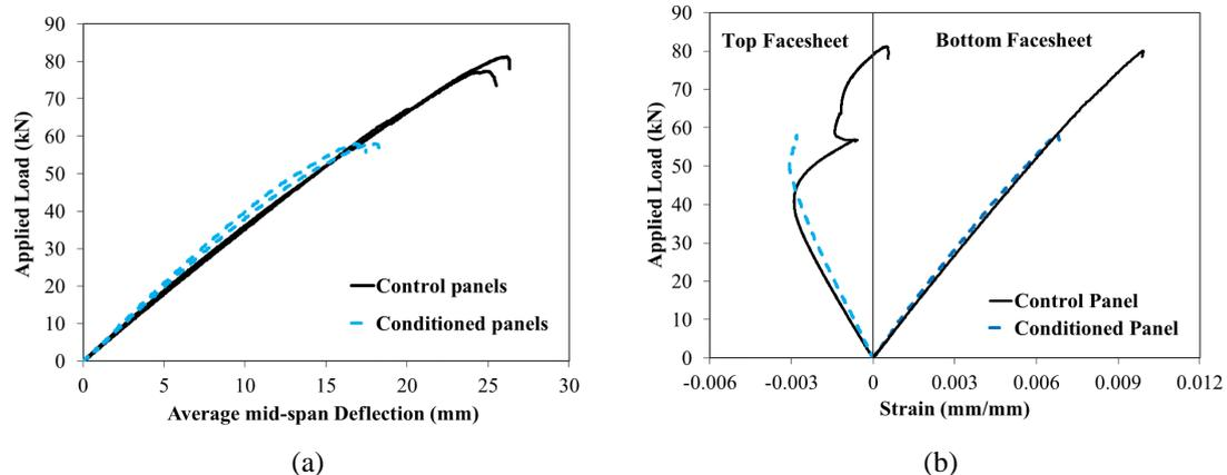
Figure 4. Test results: (a) applied load vs. mid-span deflection, and (b) applied load vs. mid-span strain.
