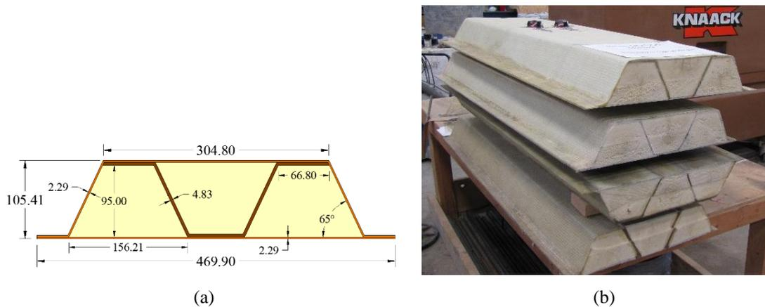
Figure 1. Mid-scale PU sandwich panels: (a) schematic of panel cross section, and (b) four prototype panels.
