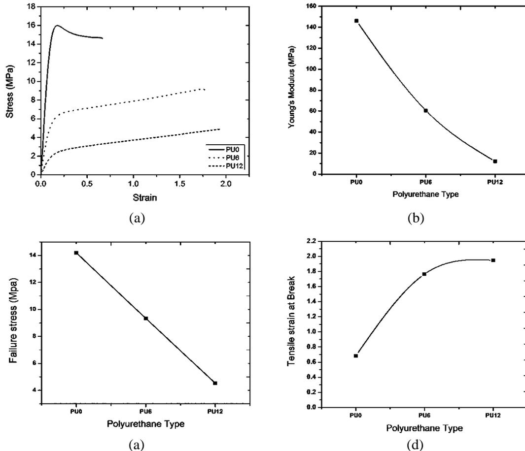
Figure 4. The tensile mechanical characteristics of the three PU samples: (a) Stress-strain curve; (b) Young's modulus; (c) Tensile stress at rupture; and (d) Strain at rupture.
