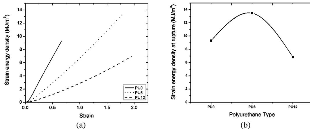
Figure 4. The tensile mechanical characteristics of the three PU samples: (a) Strain energy density vs. strain; (b) Strain energy at failure.
