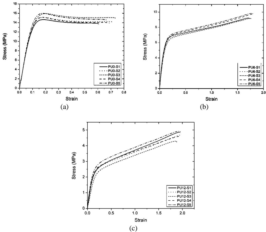
Figure 2. The engineering stress-strain curves of: (a) PU0 samples; (b) PU6 samples; and (c) PU12 samples.
