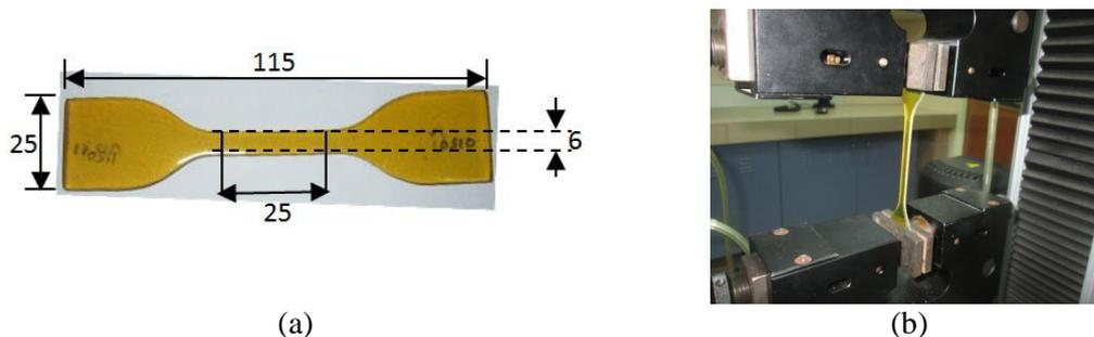
Figure 3. The: (a) Dimensions of specimens (in mm) prepared for the uniaxial tensile test; and (b) Performance of the uniaxial tensile test.
