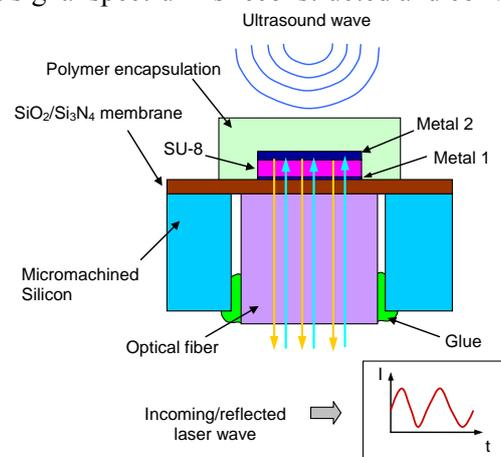
Figure 5: Acousto-optical ultrasound detector by Micro-Opto-Mechanical technology
