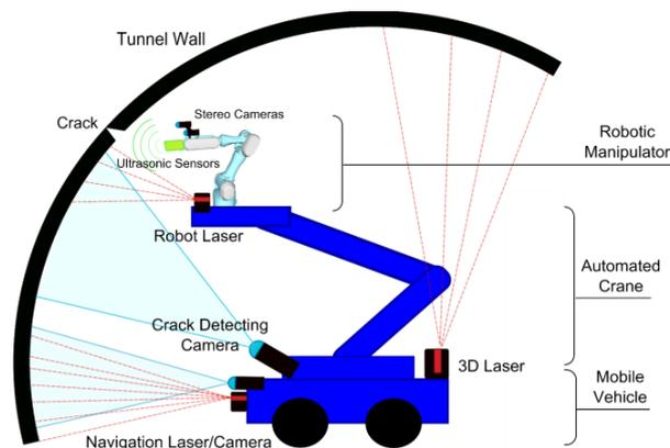
Figure 1: Conceptual design of the ROBO-SPECT system
