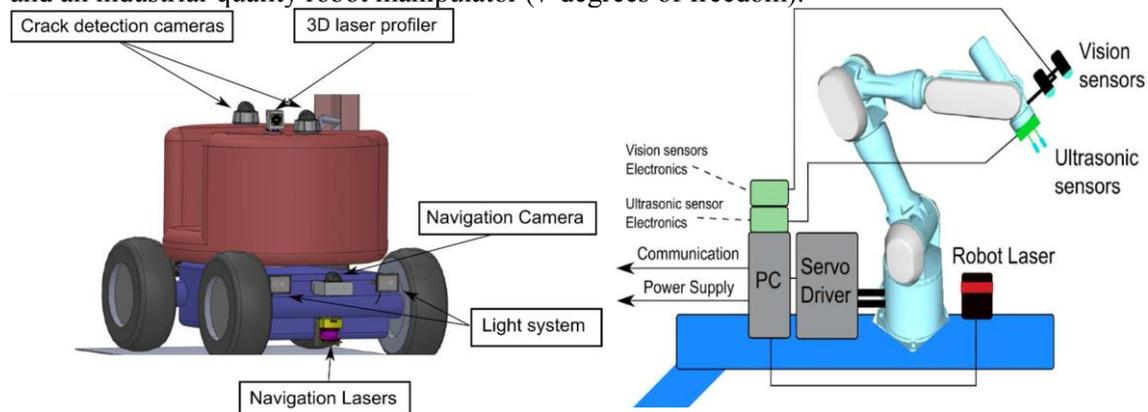
Figure 4: Mobile Vehicle System and Robotic Arm Equipment
