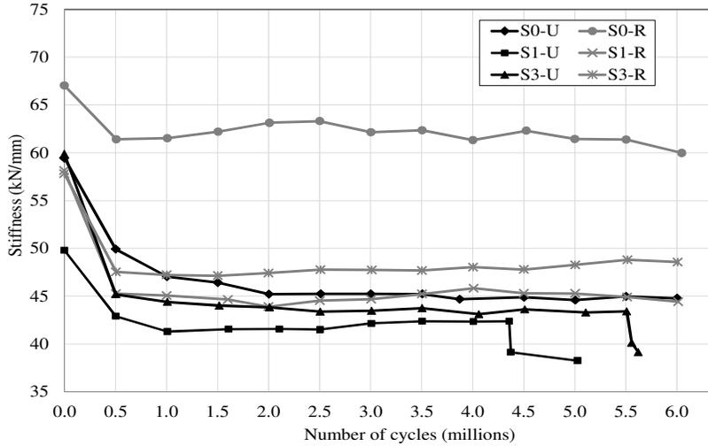
Figure 5. Stiffness at each 0.5 million increment fatigue cycles.
