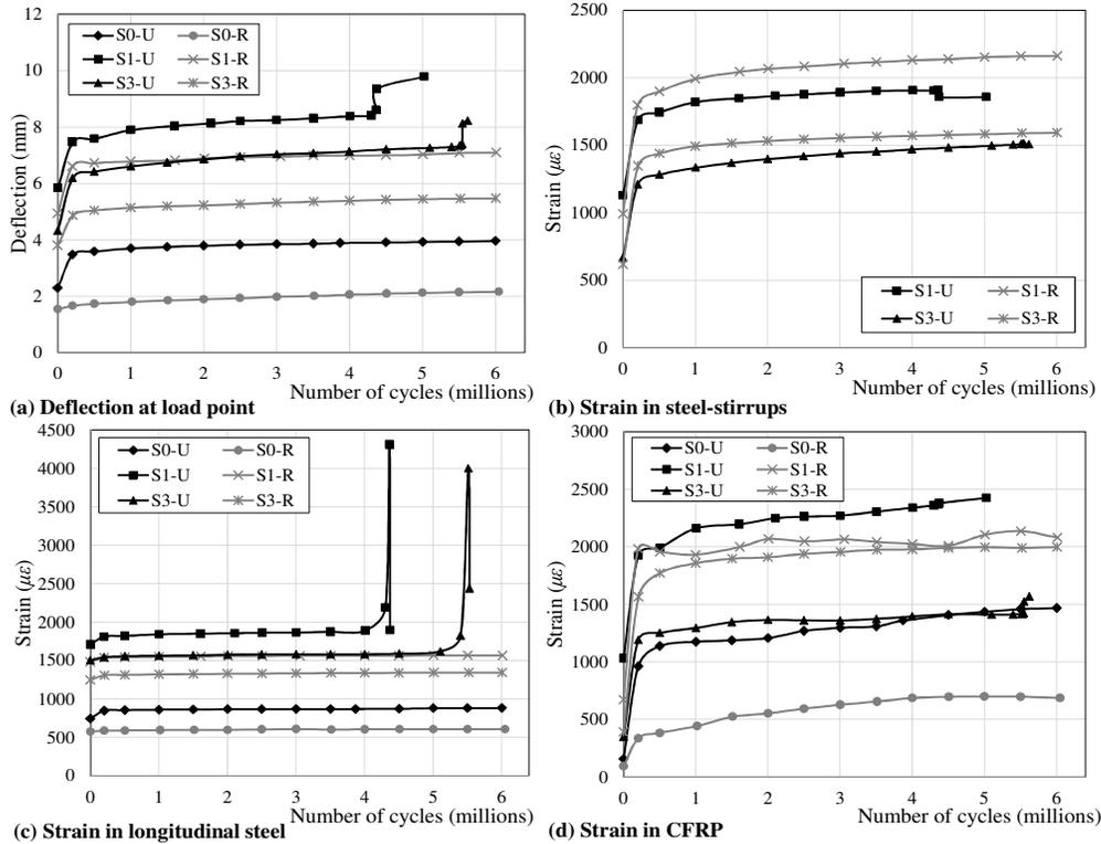
Figure 4. Deflection and strain responses versus number of cycles for  $P_{max}$ .
