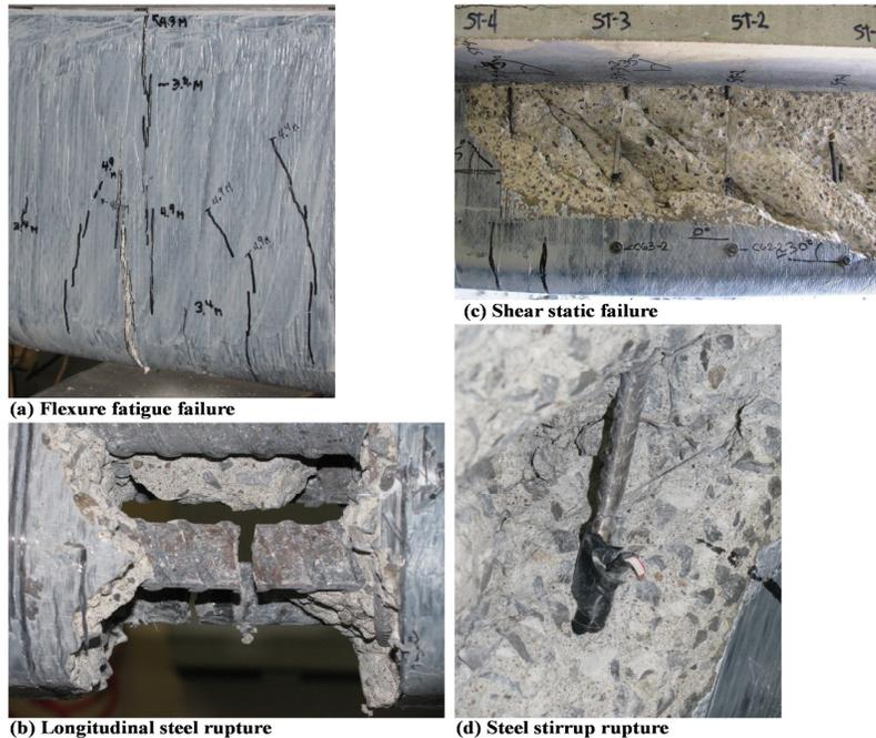
Figure 3. Failure modes under fatigue and static loading.
