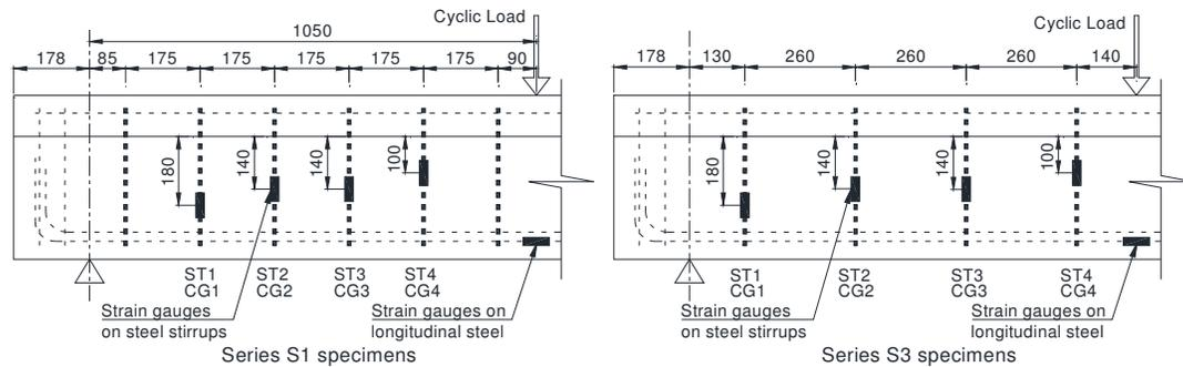
Figure 2. Test setup and instrumentation of gauges.
