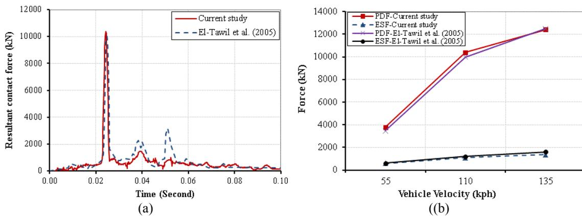
Figure 2. Current study FE results versus El-Tawil et al. (2005) FE results; (a) Impact force when vehicle's velocity was 110 kph and (b) PDF and ESF versus the vehicle velocities.
