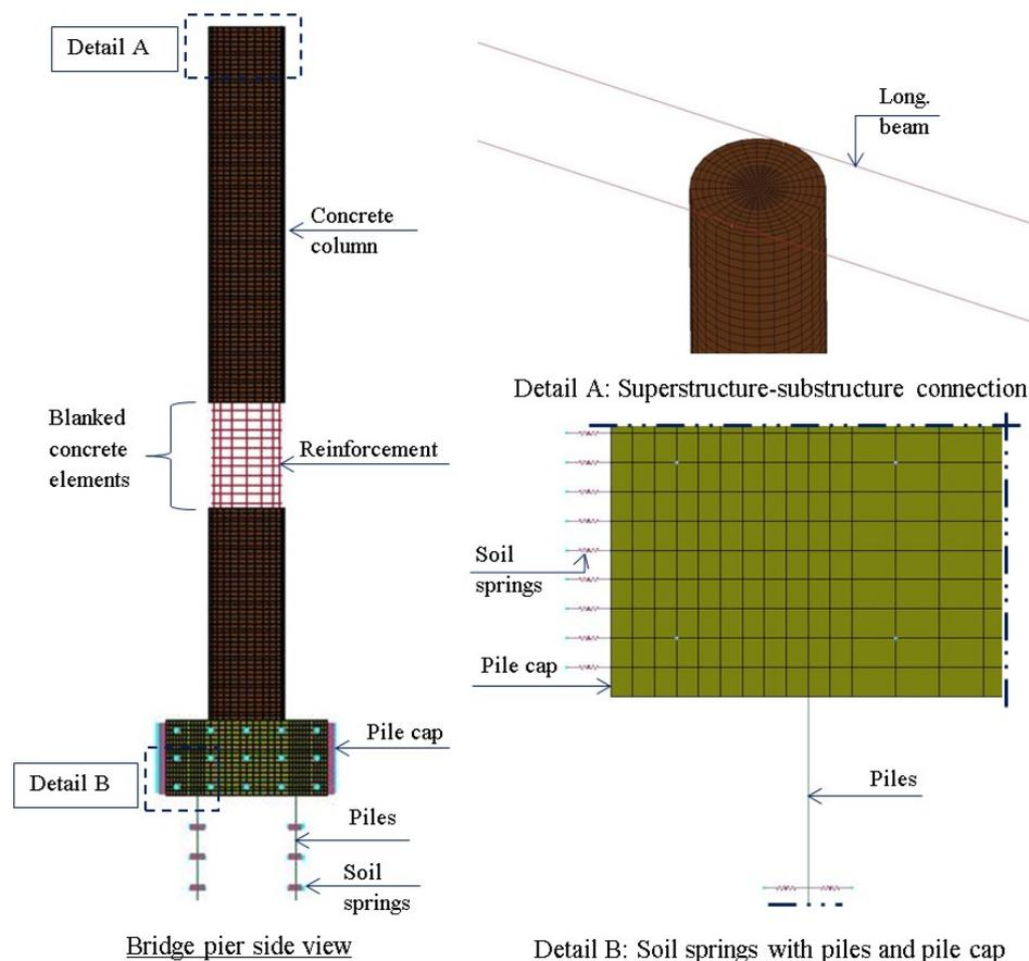
Figure 1. Components of the FE model for validation against El-Tawil's et al. results (2005)
