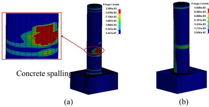
Figure 6. Column strain countour: (a) RC Column, and (b) HC-FCS column
