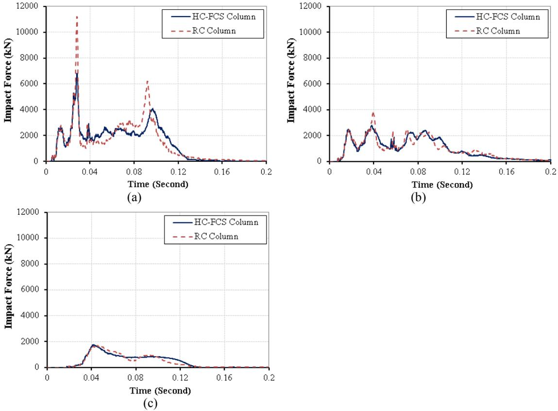
Figure 5. Time vs impact force for HC-FCS column and RC column under vehicle collision with a velocity of: (a) 112 kph, (b) 80 kph, and (c) 32 kph
