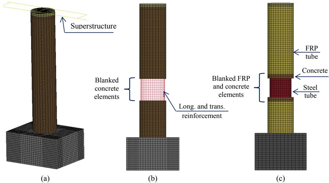
Figure 3. Columns FE modeling: (a) 3D view, (b) RC-column, and (c) HC-FCS column
