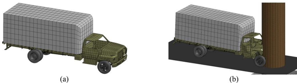
Figure 4. (a) FE model of the FORD F800-SUT and (b) Vehicle collision with the column
