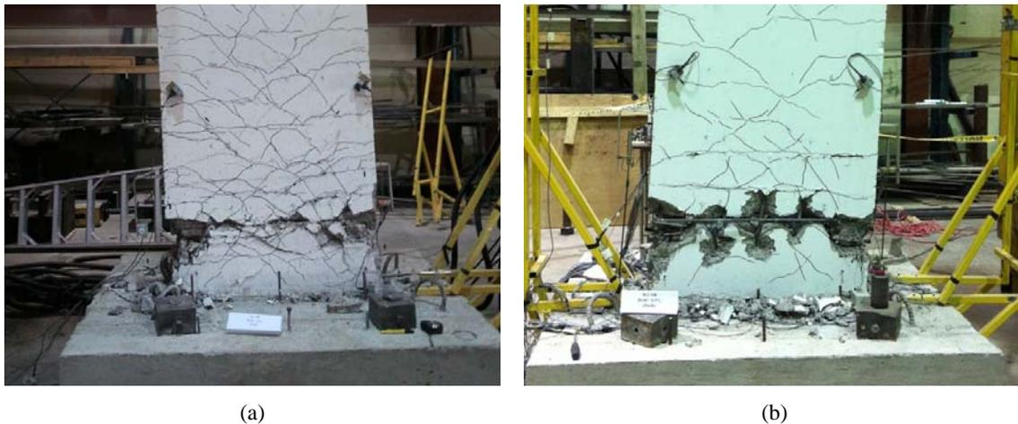
Figure 6. Condition of walls at the end of testing: a) Wall W1-SR; and b) Wall W2-NR
