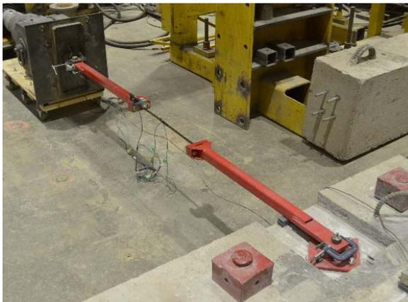
Figure 8. Proposed SMA brace subjected to cyclic loading.
