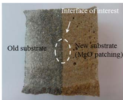
Figure 2 Specimen preparation for microscopic observation at the interface
