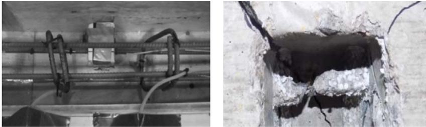
a) Embedded foam cube and the FBG sensors    b) Cut into the reinforcement bar
