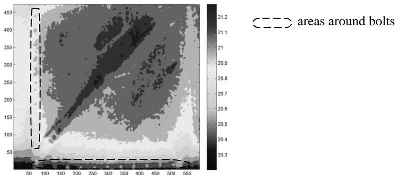
Figure 4. IR images demonstrating temperature distribution
