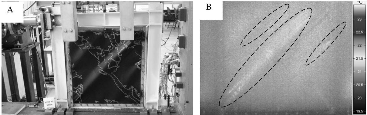
Figure 2. Heat releases at maximum 30 mm displacement in horizontal direction for HCSW-1 specimen a) shear wall photo b) IR image
