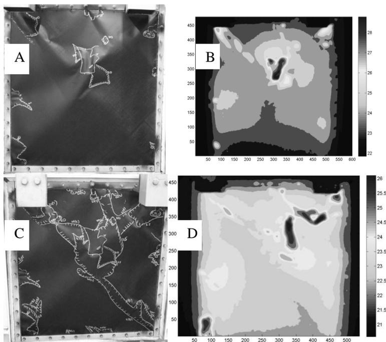
Figure 5. Delamination detection for HCSW specimen (a and b at 20 mm displacement; c and d at 25mm displacement)
