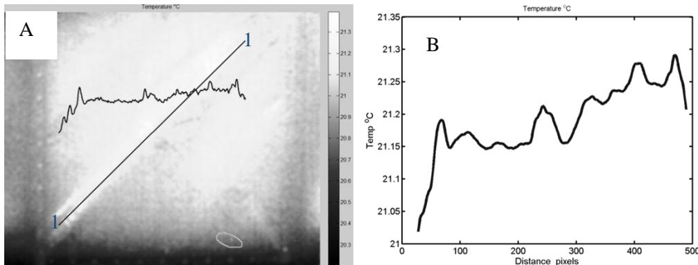
Figure 3. IR images of HCSW-1 specimen at 30 mm displacement after MATLAB processing a) temperature distribution b) tensile field profile
